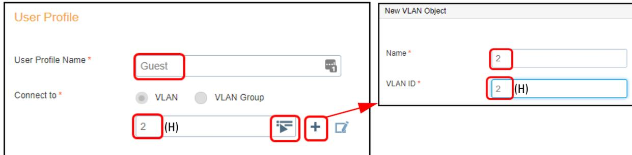
2. Select **ADD** again to obtain an Isolation User Profiles with VLAN 12 (C) using the same procedure as in the previous step.
