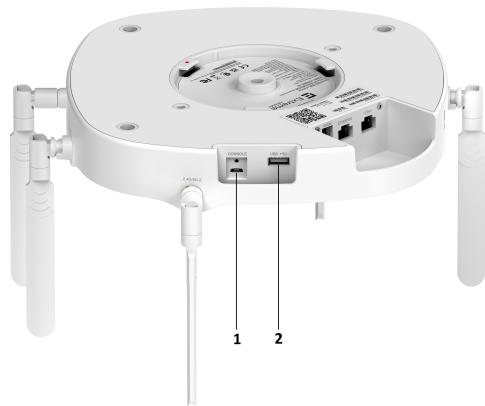
Figure 9: Front Ports and Connectors
