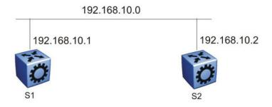
Figure 22: Example 1: OSPF on one subnet in one area
