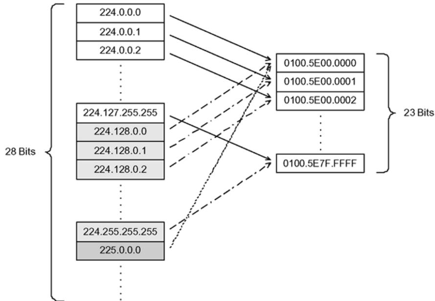
**Figure 65: Multicast IP address to MAC address mapping**
