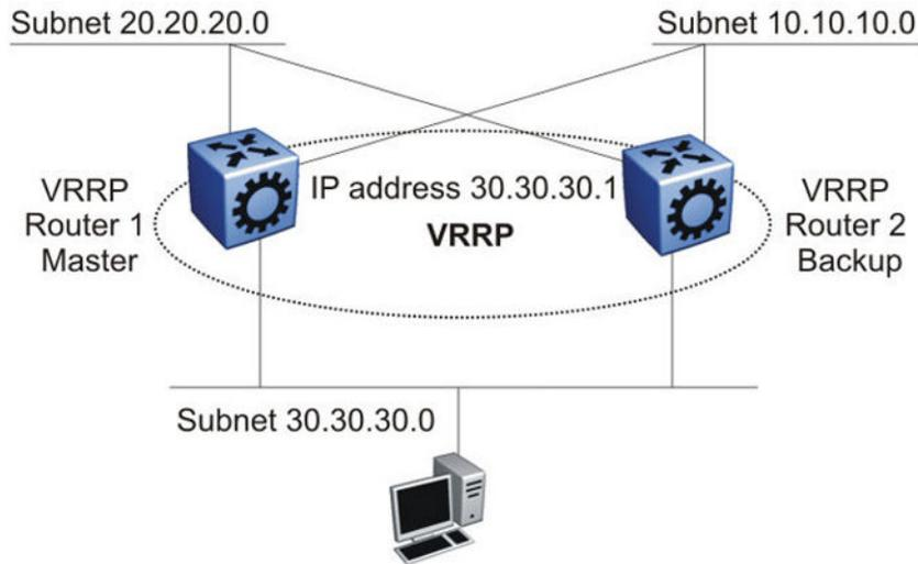
Figure 32: Avoiding excessive ICMP redirect messages without SMLT
