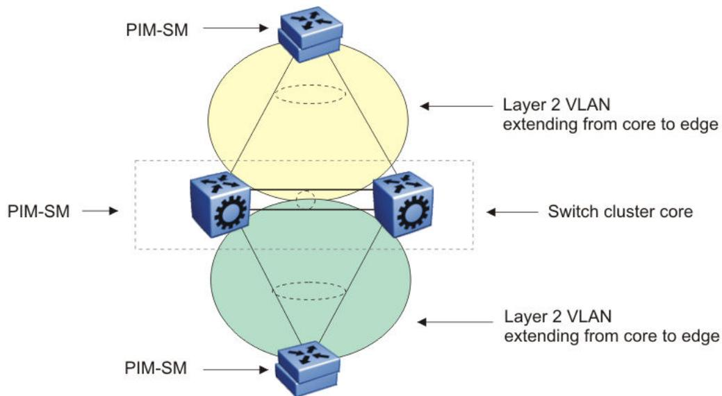
**Figure 19: Multicast SMLT triangle**
