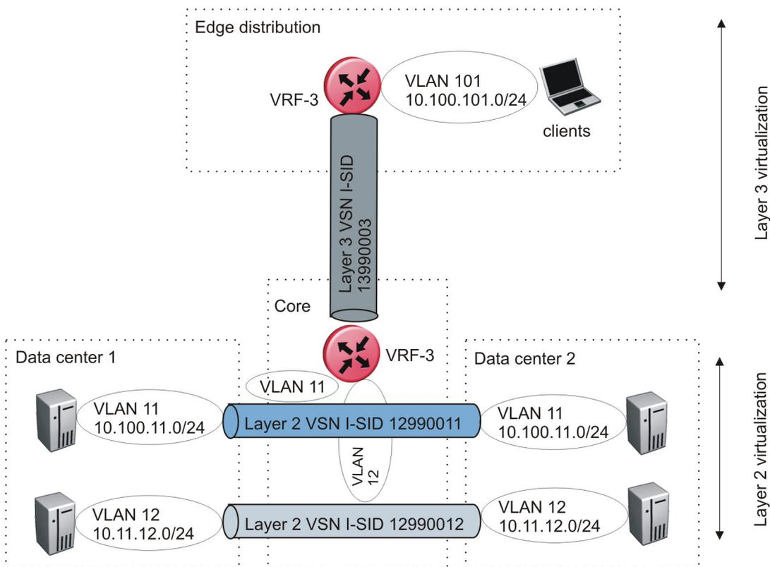
**Figure 52: VRF scenario to move traffic between data centers**
