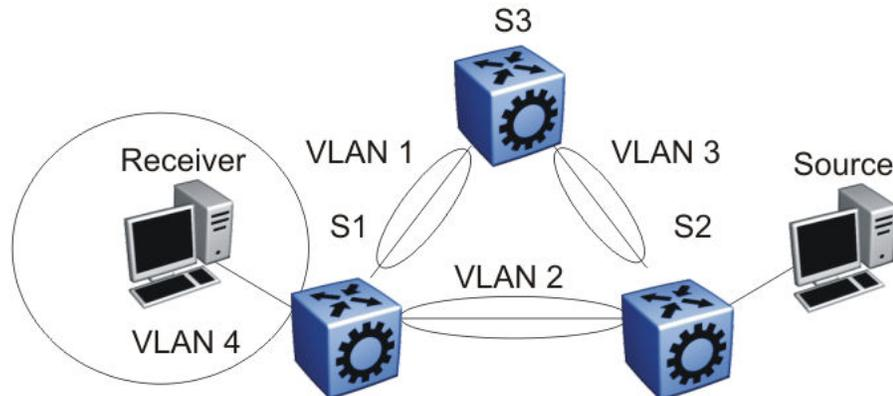
**Figure 64: IP multicast sources and receivers on interconnected VLANs**
