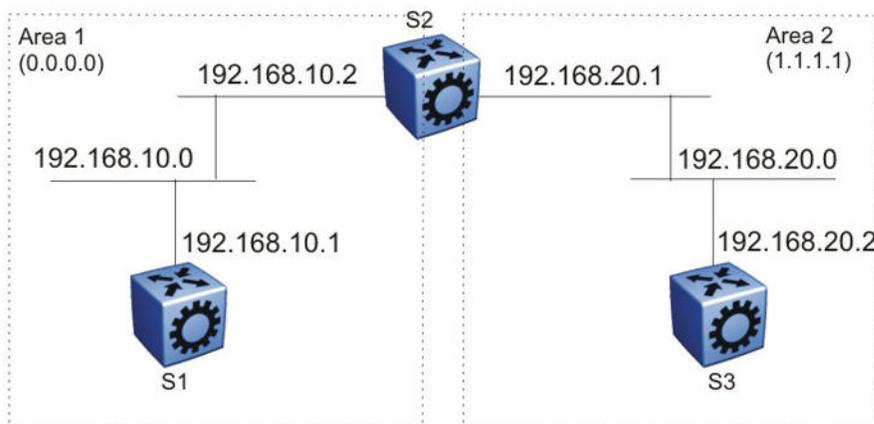
**Figure 35: Example 3: OSPF on two subnets in two areas**
