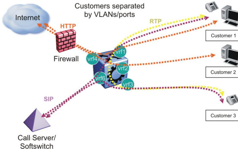
Figure 27: Inter VRF communication, internal inter-VRF forwarding
