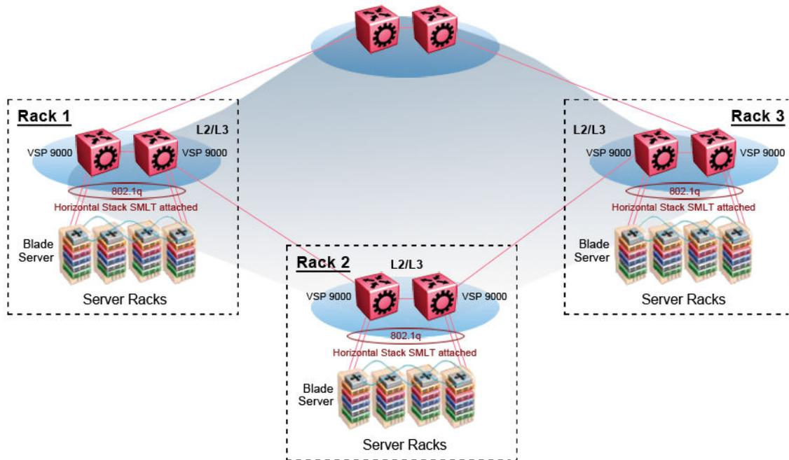
Figure 47: SPBM ring topology with shared data centers
