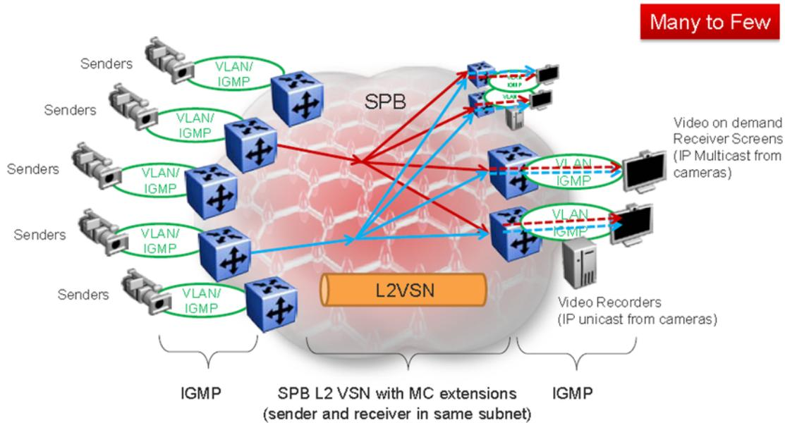
**Figure 61: Deployment scenario — bridged video surveillance and IP camera deployment for transportation, airports, and government**
