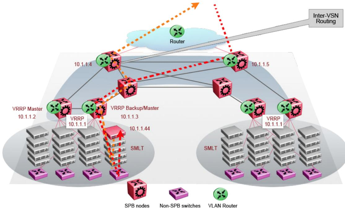
**Figure 57: Optimized routing before moving VMs**
