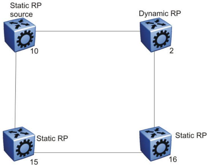
**Figure 70: Unsupported static RP configuration**
