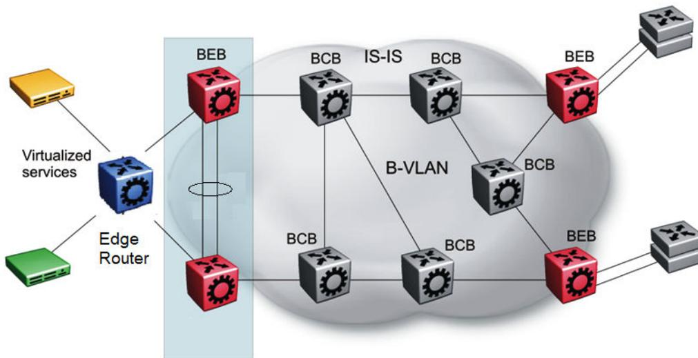
Figure 43: SPBM basic architecture
