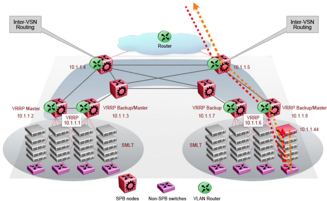
Figure 58: Optimized routing after moving VMs
