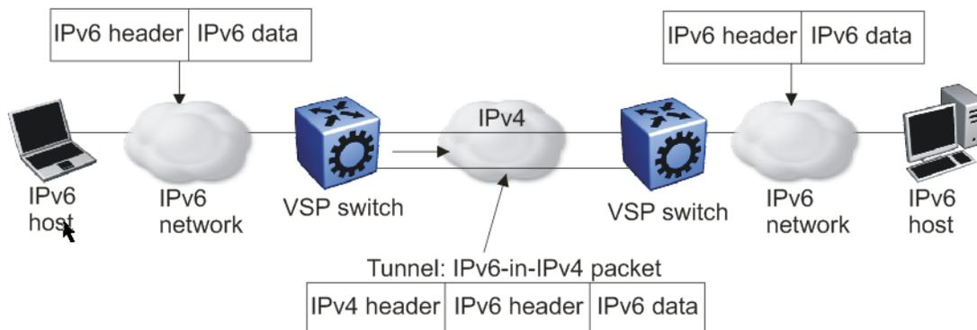
**Figure 42: IPv6 over IPv4 tunneling**
