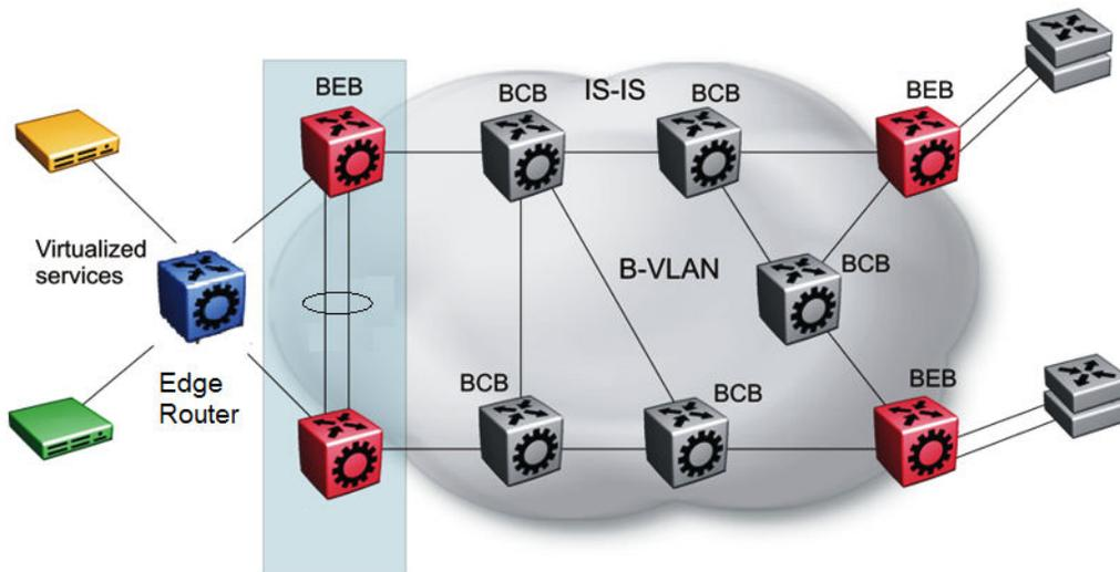
**Figure 48: SPBM basic architecture**
