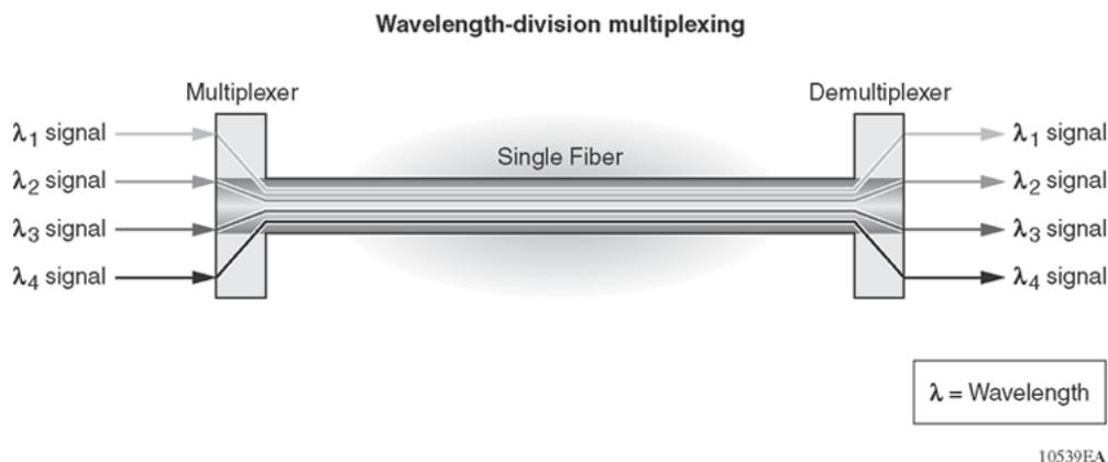
**Figure 5: Wavelength division multiplexing**
