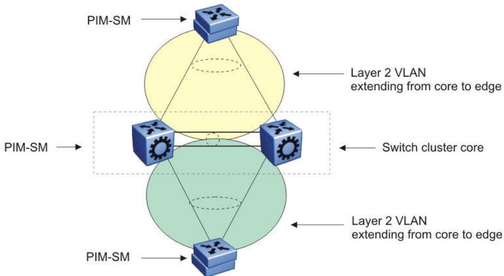
**Figure 68: Multicast SMLT triangle**
