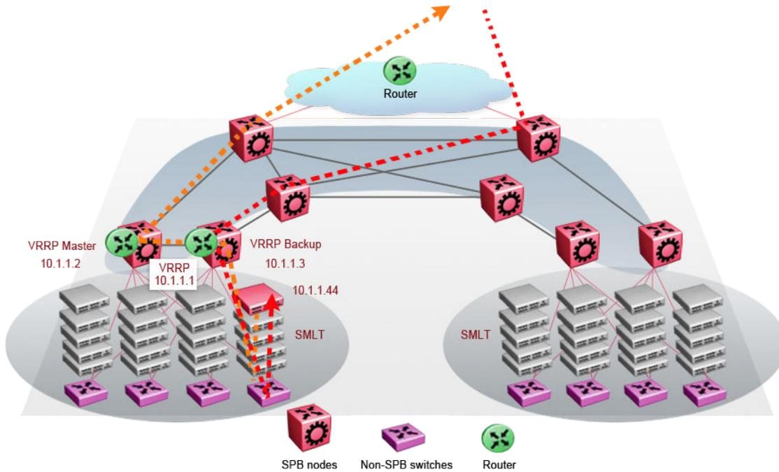
**Figure 55: Traditional routing before moving VMs**
