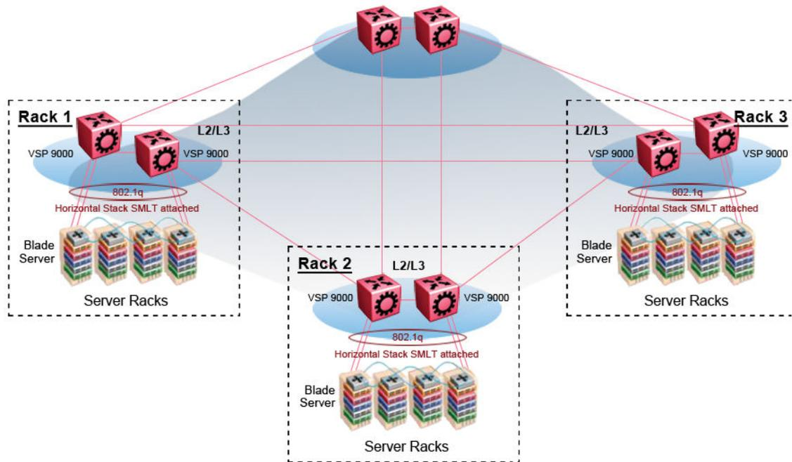
**Figure 54: SPBM data center—full mesh**
