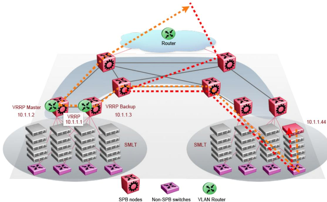
**Figure 56: Traditional routing after moving VMs**
