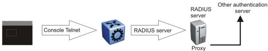
**Figure 78: RADIUS server as proxy for stronger authentication**
