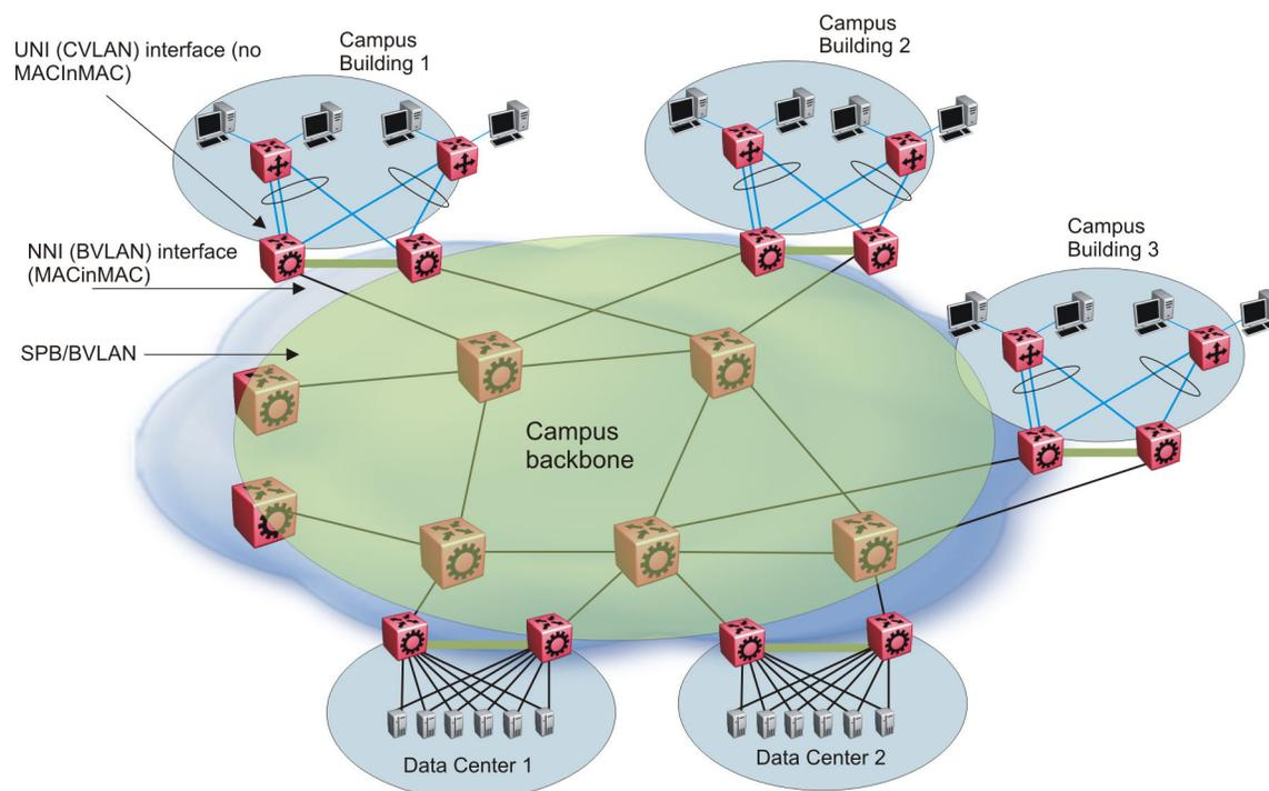
**Figure 44: SPBM support for campus and data center architecture**
