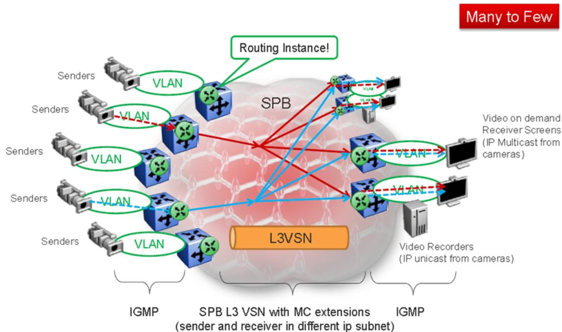
**Figure 62: Deployment scenario — Routed video surveillance and IP camera deployment for transportation, airports, and government**
