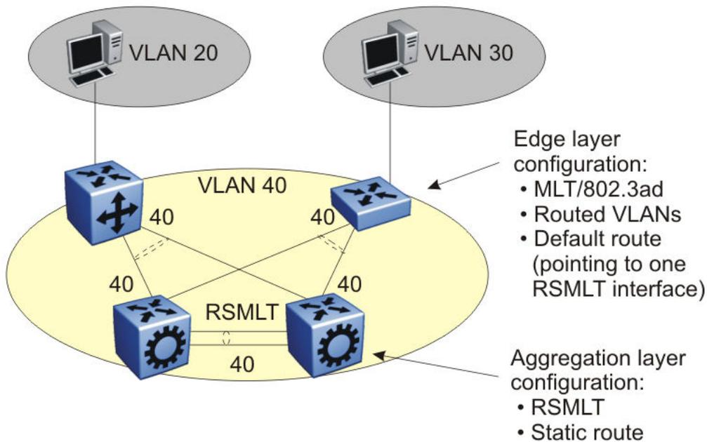
**Figure 15: VLAN edge configuration**
