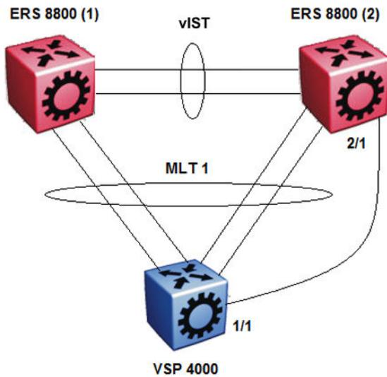
**Figure 10: VSP 4000 as an edge router and with an additional link with ERS 8800**
