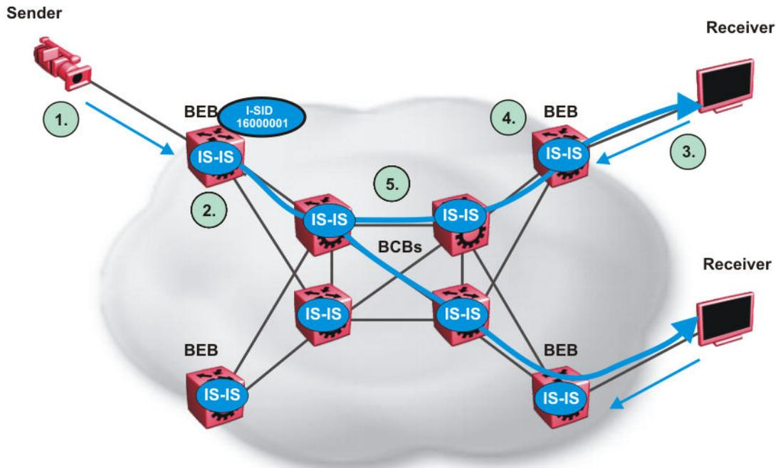
**Figure 53: IP multicast over Fabric Connect streams**
