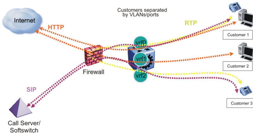
**Figure 26: Inter-VRF forwarding based on external firewall**
