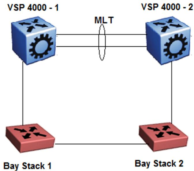
**Figure 12: Two VSP 4000 switches acting as BEBs**
