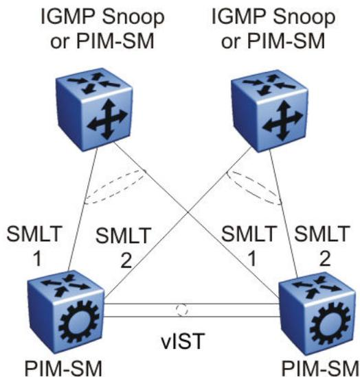
**Figure 18: Multicast routing using PIM-SM**
