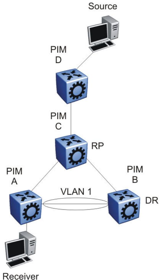
**Figure 72: Receivers on interconnected VLANs**
