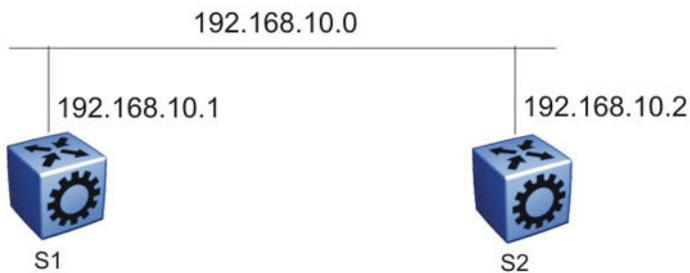
**Figure 33: Example 1: OSPF on one subnet in one area**
