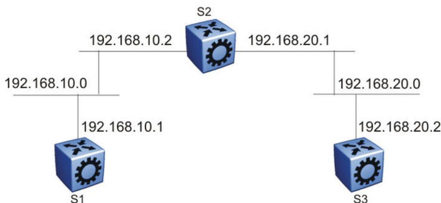
**Figure 34: Example 2: OSPF on two subnets in one area**
