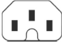
**Figure 4: IEC 60320 C16 connector**
