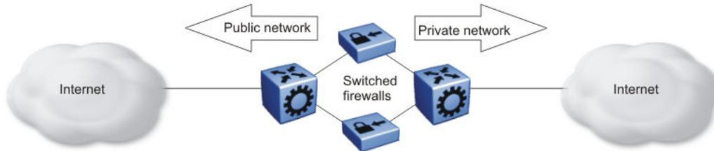
**Figure 79: Firewall load balancing configuration**
