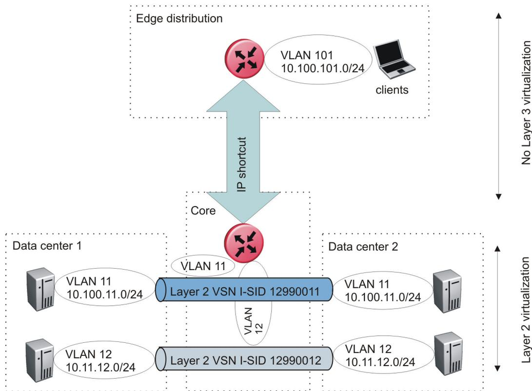
**Figure 51: IP shortcut scenario to move traffic between data centers**
