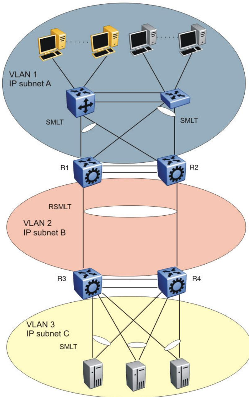
**Figure 13: SMLT and RSMLT in Layer 2 and 3 environments**
