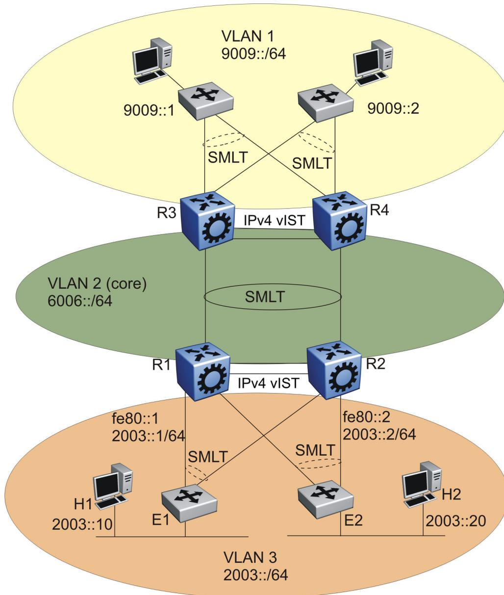
**Figure 16: IPv6 RSMLT topology**
