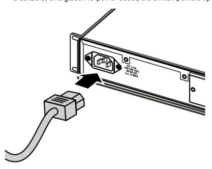
Figure 7: Connecting AC power to the back panel
