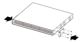
3. Slide the switch into the rack as illustrated.
