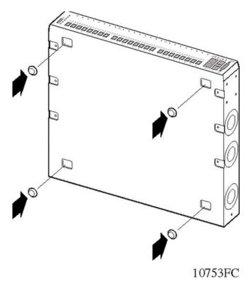
2. Set the switch on a table or shelf as illustrated below. Allow at least 2 inches (5.1 centimeters) on each side for proper ventilation and at least 5 inches (12.7 centimeters) at the back for power cord clearance.
