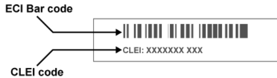
Figure 4: SFP+ bottom label
