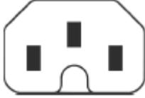
Figura 3: Conector C16 IEC 60320
