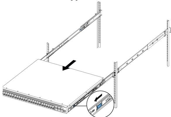
3. While the person standing in back of the chassis slides both of the white release locks (one on each side of the chassis) towards the front, the person standing in front of the chassis
