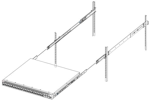
b. Pull the blue locks on the chassis rails towards the front and slide the switch into the frame.
