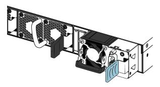
3. Verify that the power supply is fully seated in the slot. The spring latch should engage and return to its original position.
