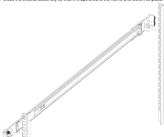
d. Close the bracket assembly so that it wraps around the frame and locks into place.
