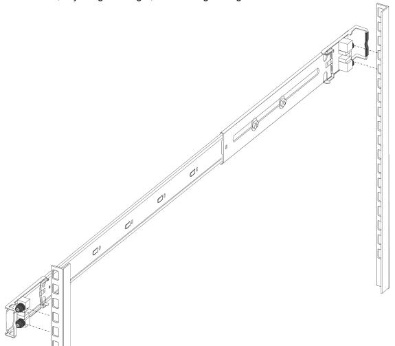
c. Push the end of the front bracket assembly so it opens up.
