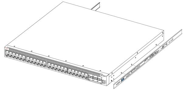
b. Slide the chassis rail to the rear until the rail locks into the standoffs.
