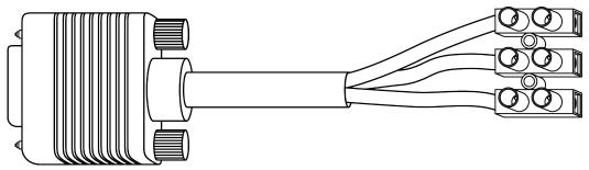
b. Refer to the tag attached to the DC power supply wiring assembly to insert the cables into their appropriate connectors.
