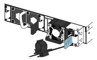
3. Verify that the power supply is fully seated in the slot. The spring latch should engage and return to its original position.
