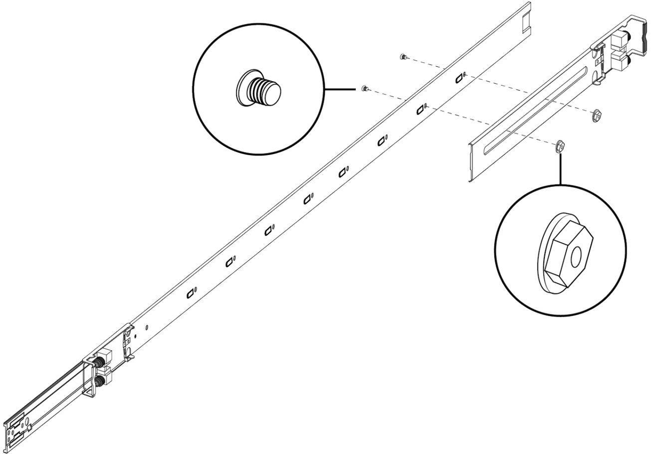
6. Use the bag with 10 countersink screws and following steps to attach the supporting plates to the rack rails:
