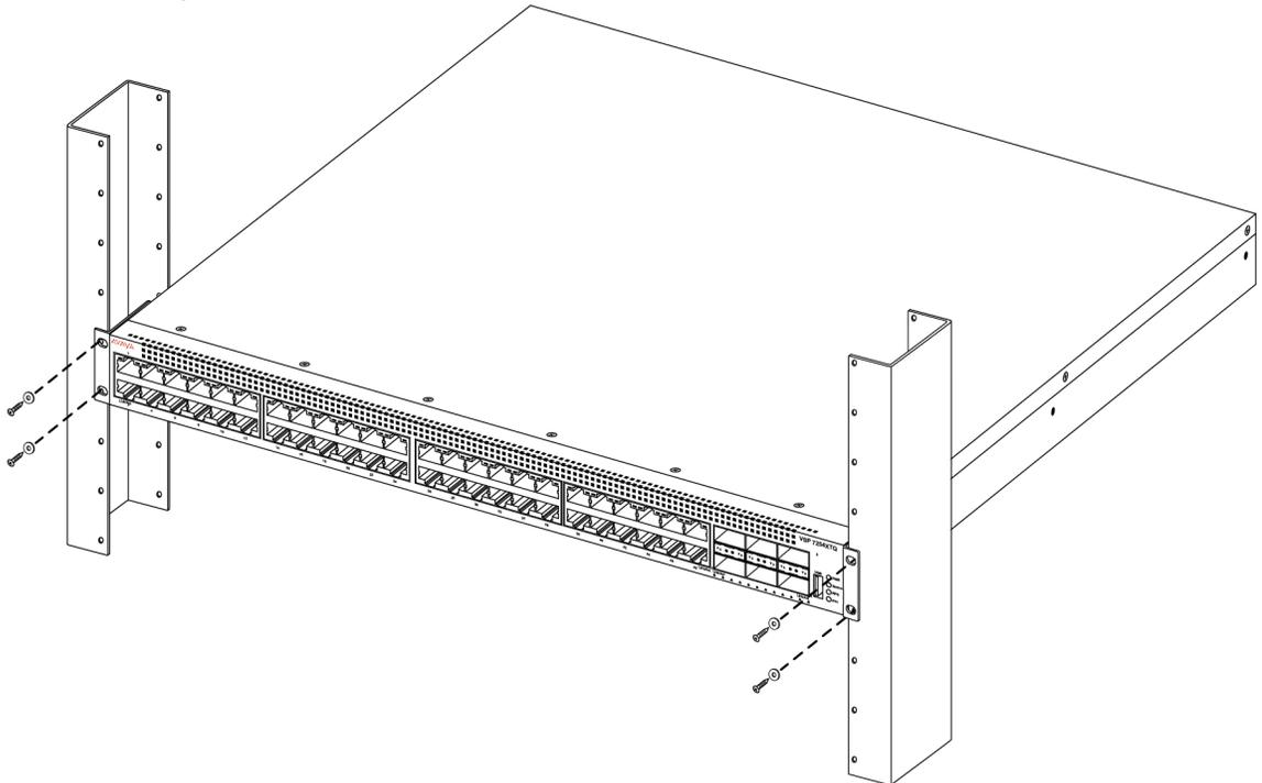
5. Verify that the switch is securely fastened to the rack.
