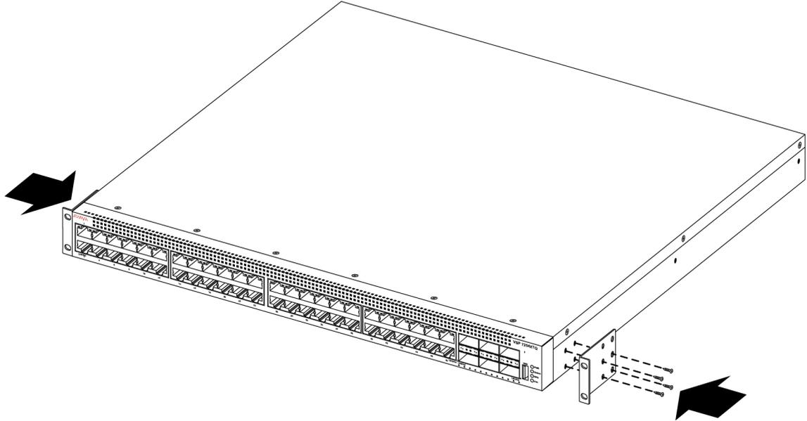
3. Slide the switch onto a shelf or tray in the rack.
