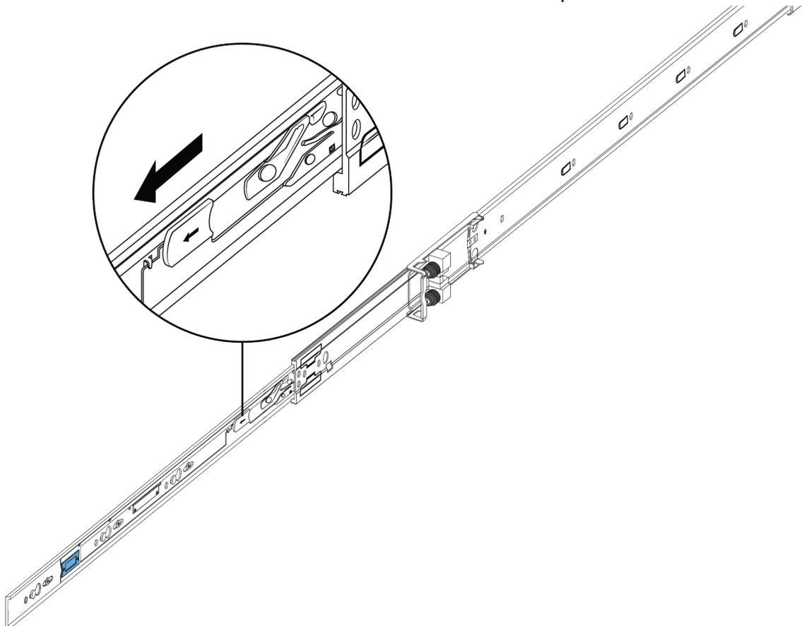
3. Lift the locking mechanism on the rack rail to slide the outer section back into the main
