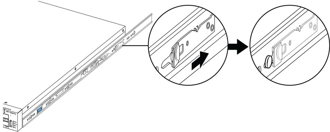
5. Use the following steps to secure the rack rails to the frame:
