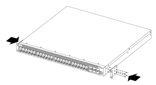
3. Slide the switch onto a shelf or tray in the rack.
