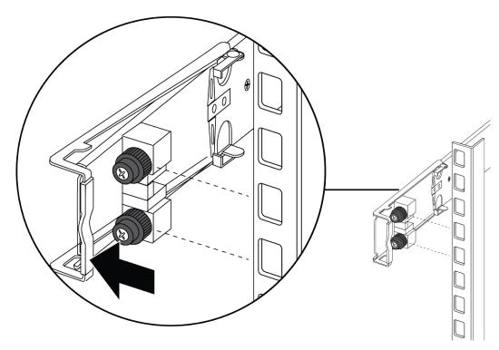
d. Insert the bracket pins into the desired holes in the frame.
