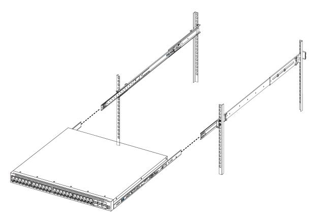
b. Pull the blue locks on the chassis rails towards the front and slide the switch into the frame.
