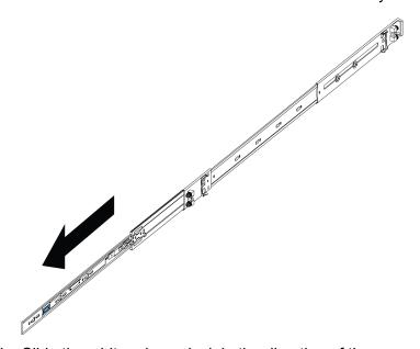
b. Slide the white release lock in the direction of the arrow stamped on the lock.
