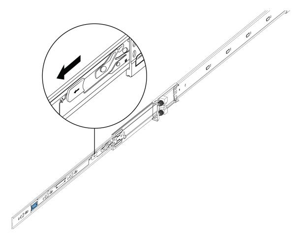
3. Lift the locking mechanism on the rack rail to slide the outer section back into the main section.
