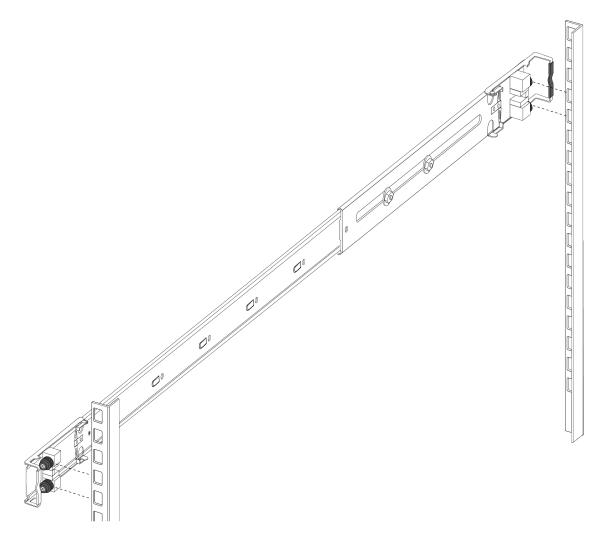
c. Push the end of the front bracket assembly so it opens up.
