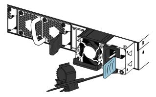
3. Verify that the power supply is fully seated in the slot. The spring latch should engage and return to its original position.
