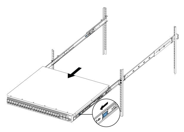
3. While the person standing in back of the chassis slides both of the white release locks (one on each side of the chassis) towards the front, the person standing in front of the chassis pulls the chassis out of the rack.
