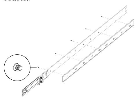
7. Insert the long rack rail bracket into the supporting plate.
