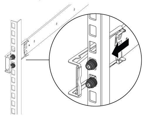
e. Close the bracket assembly so that it wraps around the frame and locks into place.
