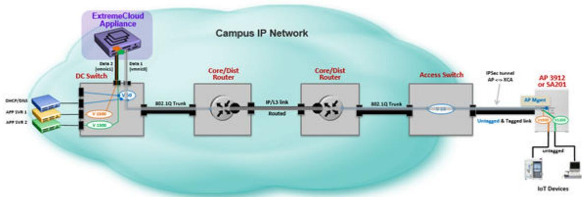
**Figure 16: Topology using local VLAN attachment with Bridged@AC**
