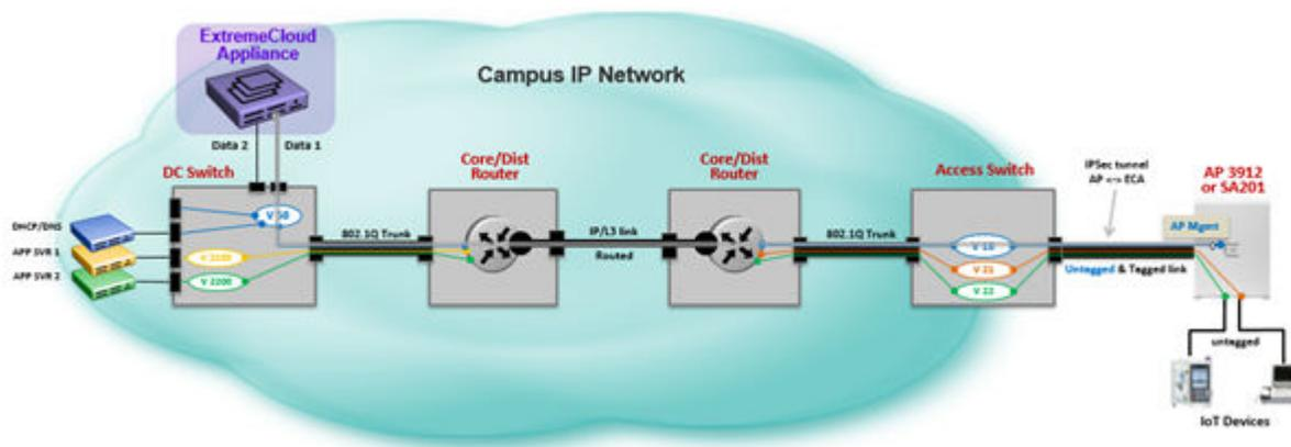
**Figure 13: Topology using local VLAN attachment with Bridged@AP**
