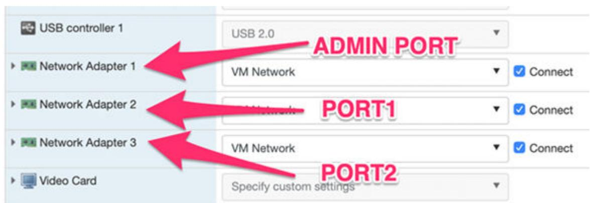
**Figure 10: VMWare: Network Adapters connected to ExtremeCloud Appliance**
