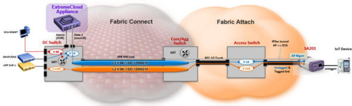
Figure 18: Topology using Fabric Attach mode
