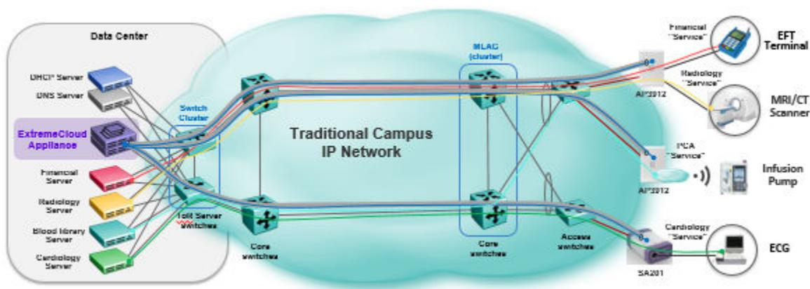
**Figure 2: Local VLAN Attachment model**
