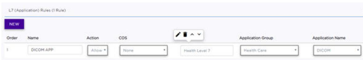
**Figure 28: ExtremeCloud Appliance Layer 7 rule configuration**
