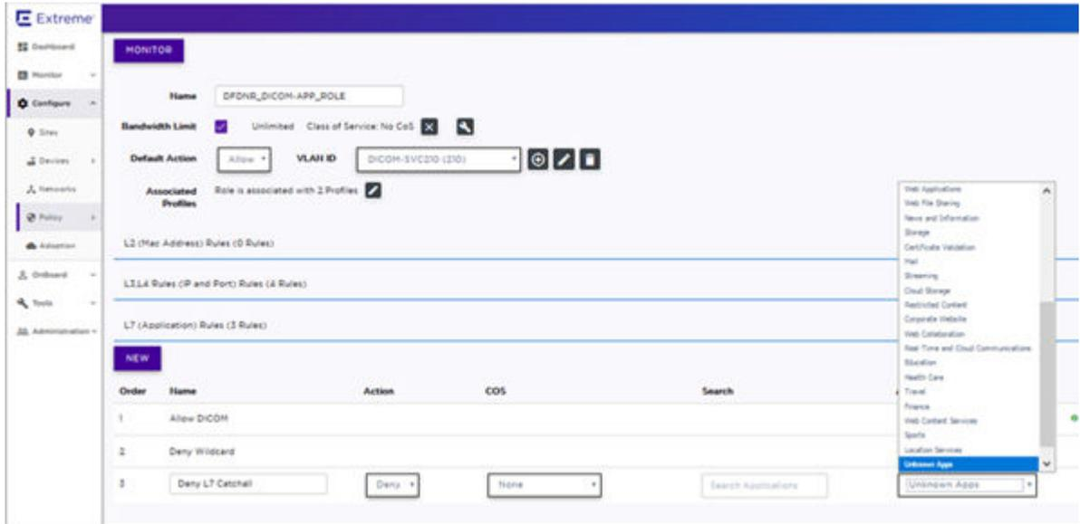
**Figure 30: ExtremeCloud Appliance DICOM role with Layer 7 Unknown Apps rules**
