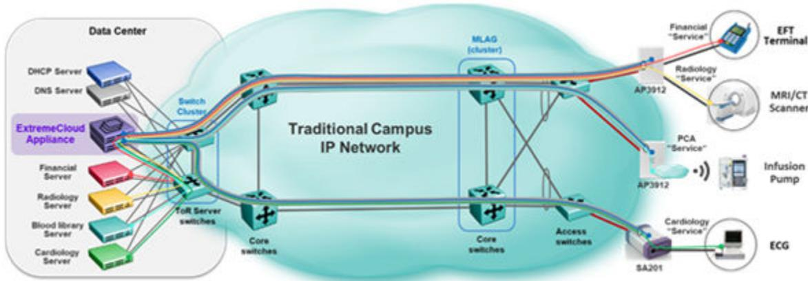
Figure 3: IPsec Tunnel Overlay model
