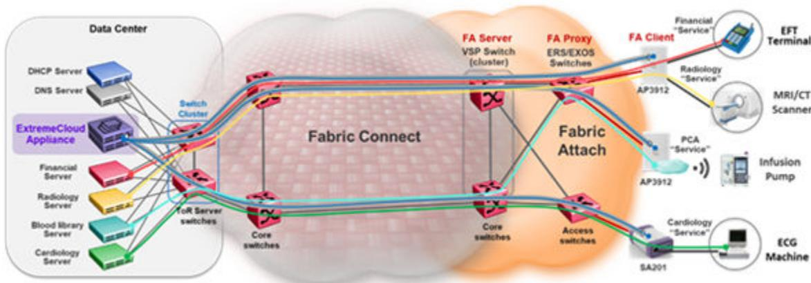
Figure 4: Fabric Connect with Fabric Attach model
