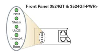
Figure 10: ERS 3524 Front Panel LEDs
