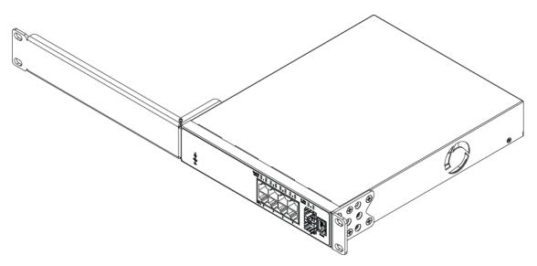
4. Slide the switch into the rack as shown in the figure that follows. Insert and tighten the rack mount screws.
