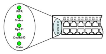
Figure 12: ERS 3549GTS/GTS-PWR+ Front Panel LEDs
