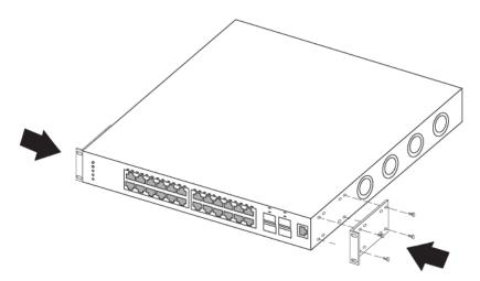
3. Slide the switch into the rack. Insert and tighten the rack mount screws.
