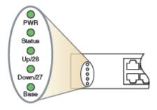
Figure 11: ERS 3526 Front Panel LEDs
