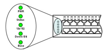
Figure 13: ERS 3550T/T-PWR+ Front Panel LEDs
