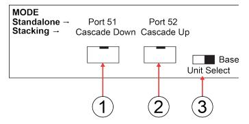
Figure 6: ERS 3550T and ERS 3550T-PWR+ rear ports
