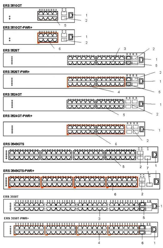
Figure 1: ERS 3500 series front panel port illustrations
