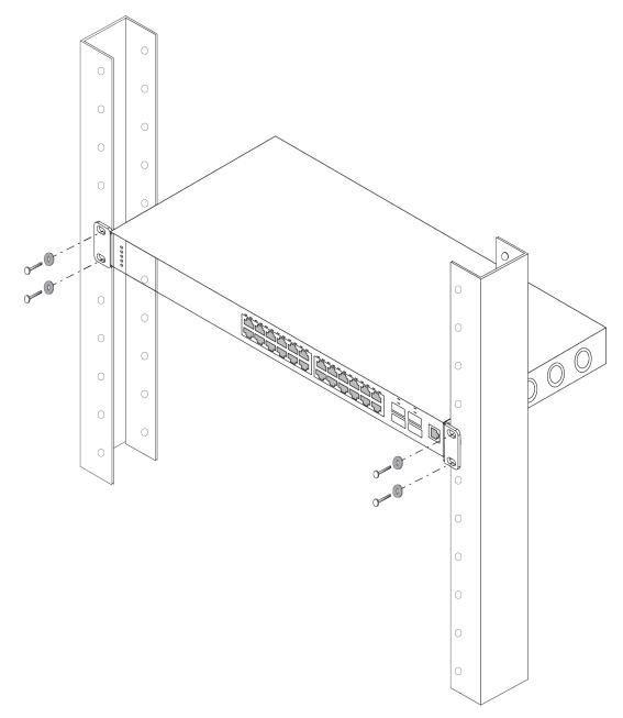
4. Verify that the switch is securely fastened to the rack.
