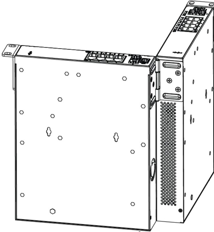
3. Attach the standard rack mount bracket ears to the outer end of each switch as shown below.
