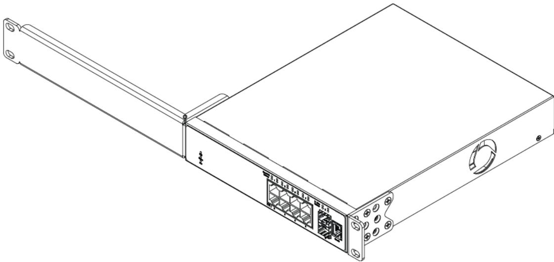
4. Slide the switch into the rack as shown in the figure that follows. Insert and tighten the rack mount screws.
