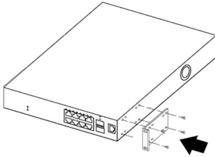
3. With the front of the ERS 3510GT or ERS 3510GT-PWR+ unit facing you, attach the long bracket from the optional kit (see Figure that follows) to the left side of the switch using the flathead screws provided.
