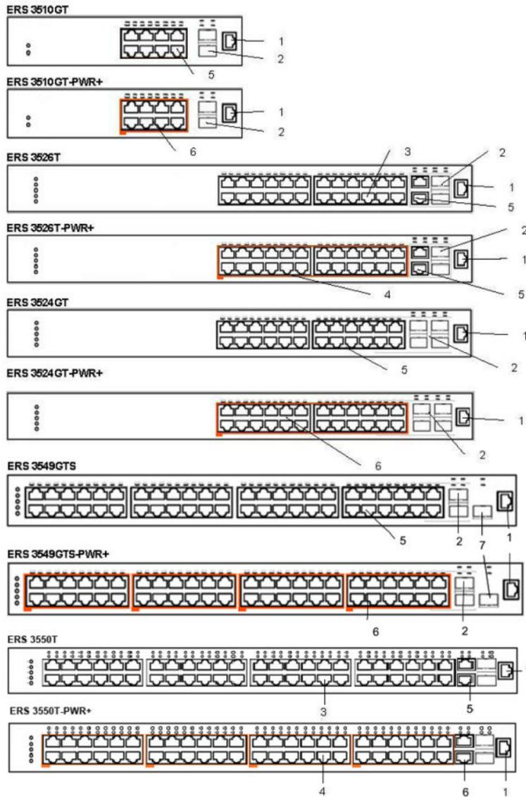
Figure 1: ERS 3500 Series front panel illustrations
