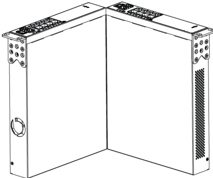
4. After the switches are joined together, fold the hinged bracket inward.
