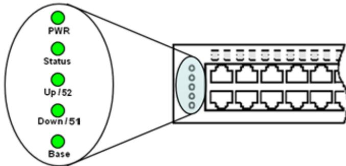
**Figure 13: ERS 3550T/T-PWR+ Front Panel LEDs**
