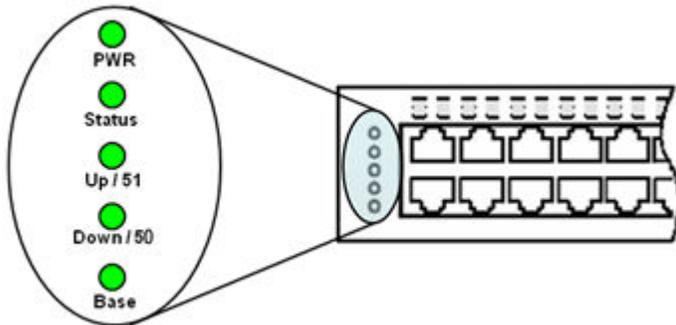
**Figure 12: ERS 3549GTS/GTS-PWR+ Front Panel LEDs**
