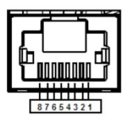
Figure 6: RJ45 console port pin-out
