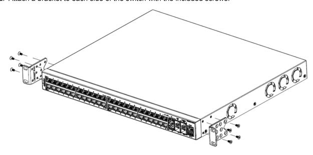
3. Slide the switch into the rack. Insert and tighten the rack-mount screws.
