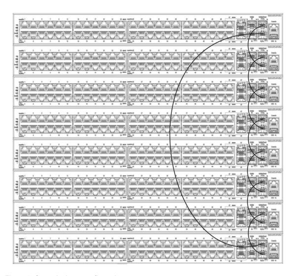
Figure 3: Cascade down configuration
