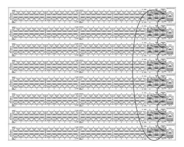
Figure 4: Cascade up configuration
