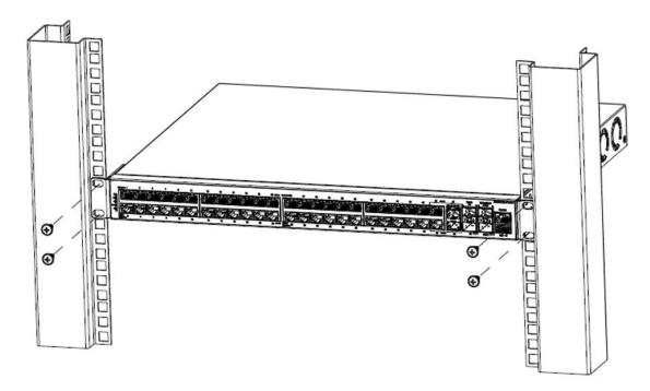
4. Verify that the switch is securely fastened to the rack.
