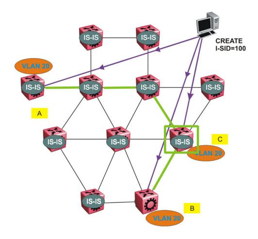
Figure 10: Shortest path tree for source node C
