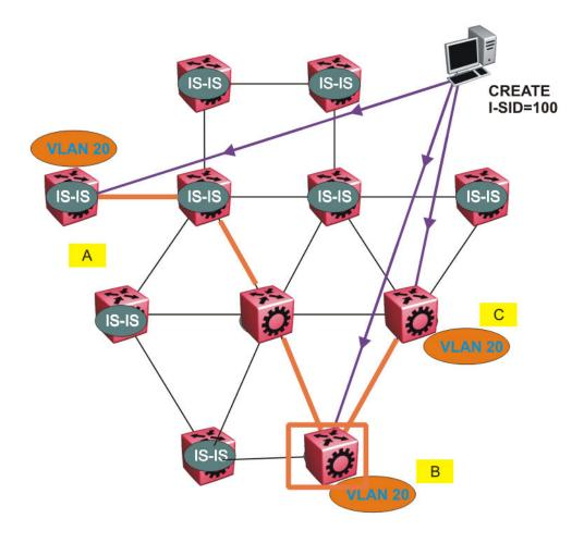
Figure 9: Shortest path tree for source node B
