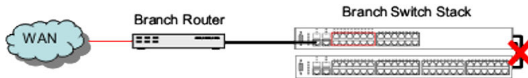
Figure 4: Remote Branch Office – Failure Scenario 3
