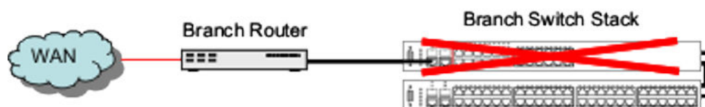
Figure 2: Remote Branch Office - Failure Scenario 1
