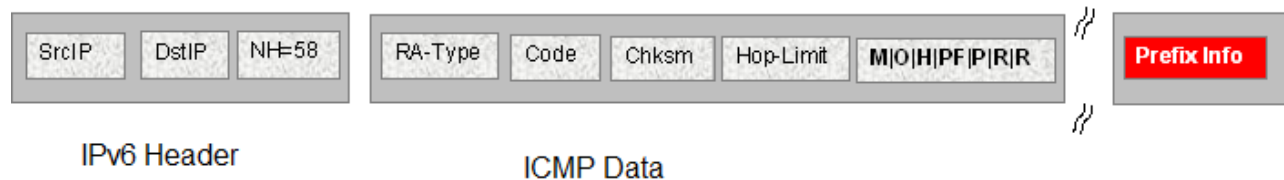
Figure 15: IPv6 ICMP RA data packet outline
