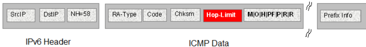
Figure 18: IPv6 ICMP RA data packet outline
