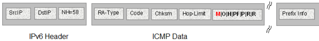
Figure 17: IPv6 ICMP RA data packet outline
