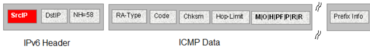
Figure 14: IPv6 ICMP RA data packet online
