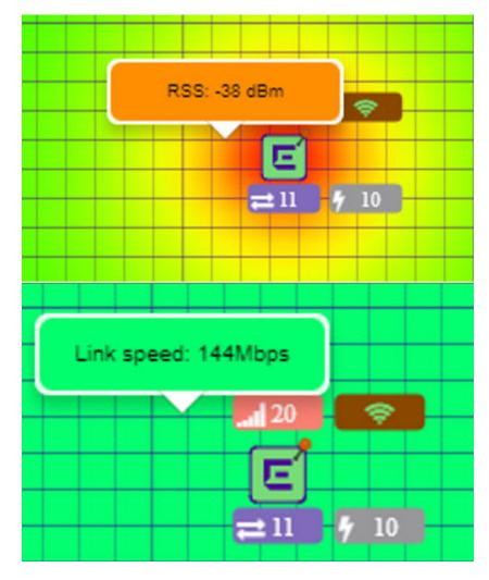
Figure 18: Push-Pin Reading for Heatmap Values
