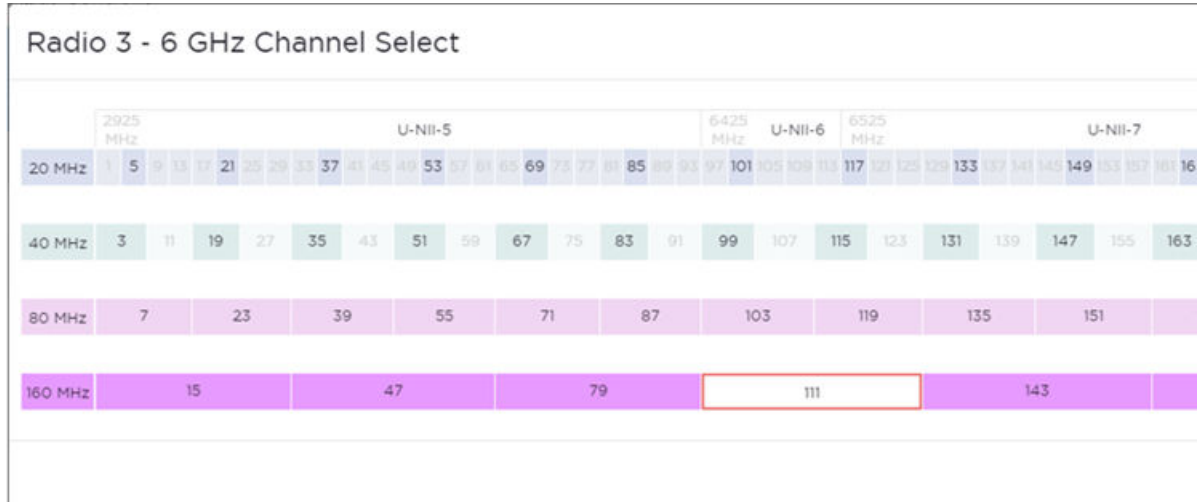
Figure 52: Channel Select dialog displaying 6 GHz band available channels
