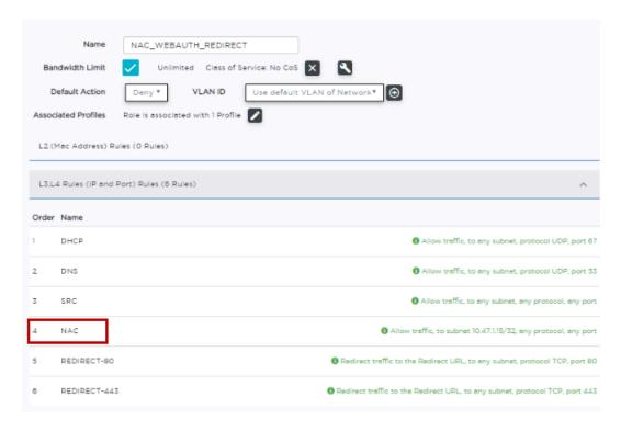
Figure 56: Example Redirection Role on ExtremeCloud IQ Controller that includes six L3/L4 rules
