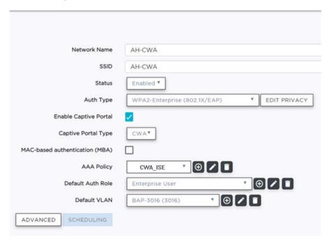
Figure 43: CWA Network on ExtremeCloud IQ Controller
