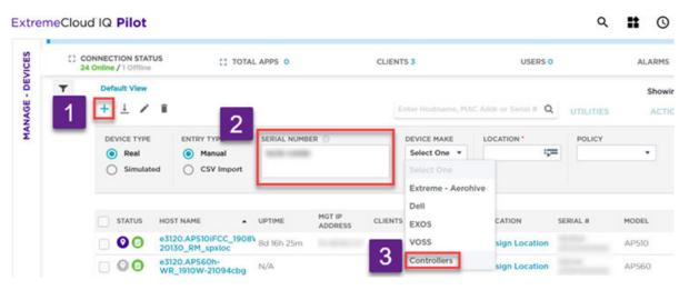
Figure 89: Manually adding a controller to ExtremeCloud IQ
