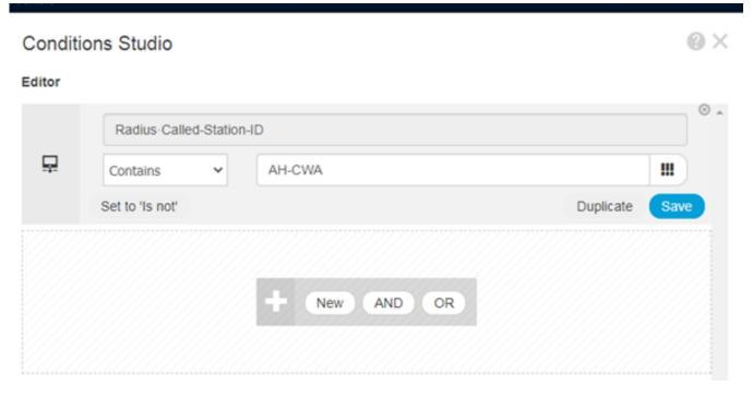
Figure 48: Condition to match on SSID
