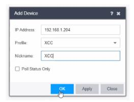
Figure 66: Add ExtremeCloud IQ Controller as a device in ExtremeCloud IQ - Site Engine
