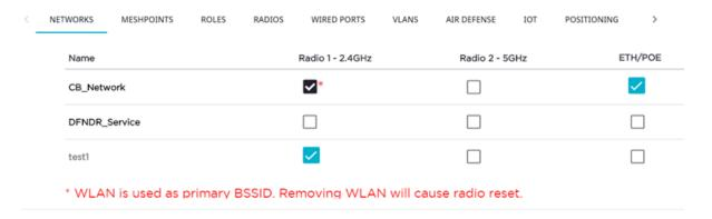
Figure 83: Configuration Profile Network Configuration – Client Bridge on a single interface AP
