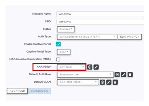
Figure 54: CWA Network on ExtremeCloud IQ Controller — ExtremeControl
