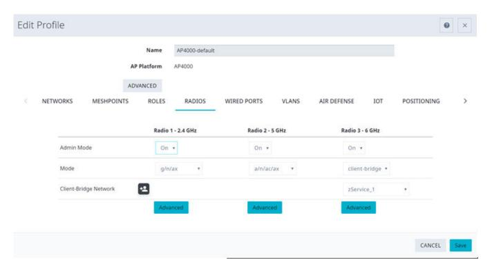
Figure 81: Configuration Profile with Client Bridge Configuration
