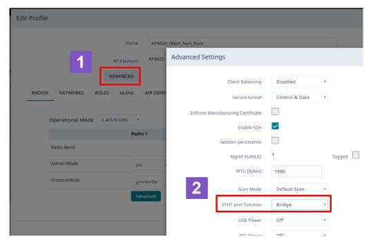
Figure 32: Configure Transparent Bridge from Device Group Configuration Profile
