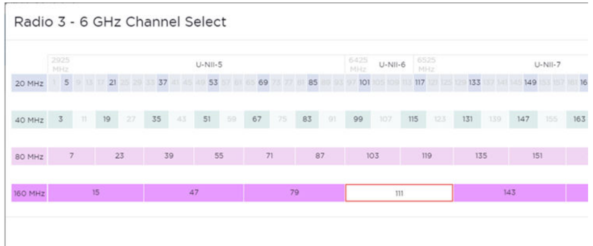
Figure 46: Channel Select dialog displaying 6 GHz band available channels
