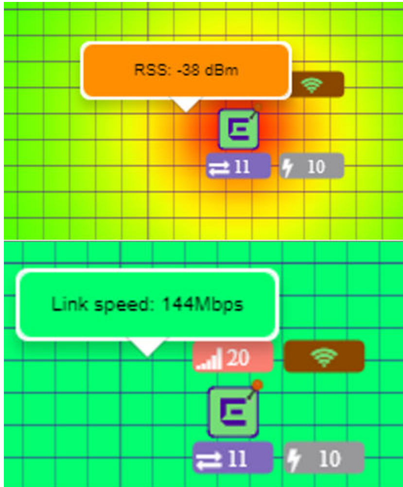
Figure 19: Push-Pin Reading for Heatmap Values
