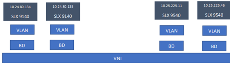
Figure 18: Scope of tenant constructs
