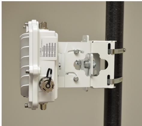
7. Use a torque wrench or a ratchet and a 10mm socket, or an adjustable wrench, to finish attaching the Access Point bracket section to the angle adapter bracket section with the M6 hex flange screws in the open slot connections and the top holes on the angle adapter bracket section. Do not tighten the screws until all rotation and tilt adjustments are complete.
