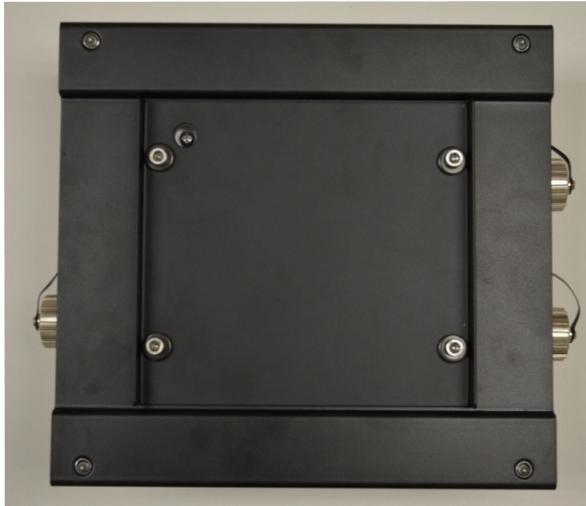
2. Using a 5mm allen wrench or box wrench, tighten the screws to 150 inch pounds (lbf-in).
