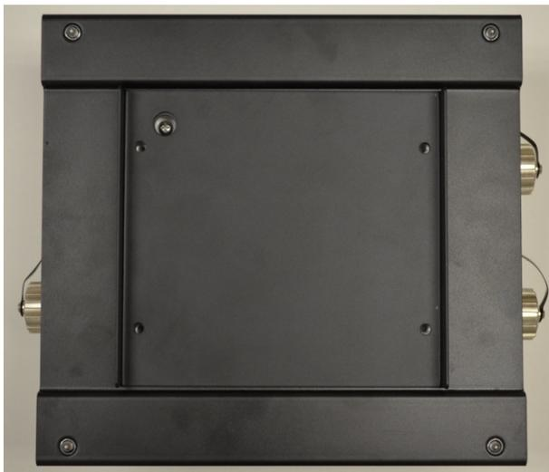
1. Insert four screws with washers through the holes of the three plates and into the screw holes on the bottom of the VMM.
