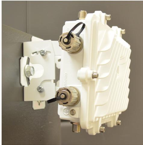
4. Use a torque wrench or a ratchet and a 10mm socket, or an adjustable wrench, to finish attaching the angle adapter bracket section to the Access Point bracket section with the four M6 hex flange screws in the open slot connections and the top holes on the angle adapter bracket section. Do not tighten the screws until all rotation and tilt adjustments are complete.
