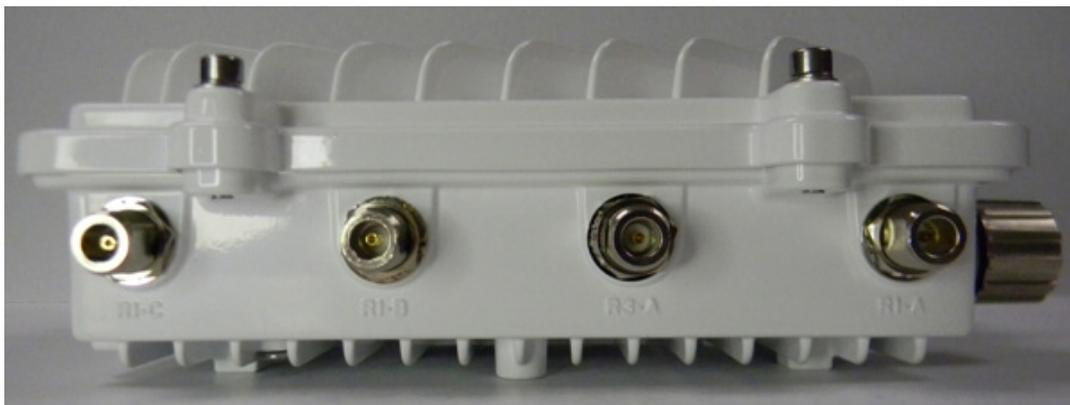
As with the two radio models, R1 ports relate to the software configured radio 1 settings. When mounting antennas to connectors marked R2-A, R2-B and R2-C, the antenna ports relate to the software configured radio 2 settings. Care must be taken to provide the correct antenna for the operating band of each port.
