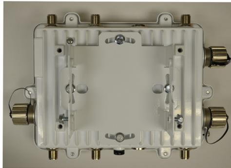
5. With the Access Point positioned so that the gore vent is facing down, insert the two M6 hex flange screws in the bottom holes on the sides of the Access Point bracket section into the open slot connections on the bottom of the angle adapter bracket section.
