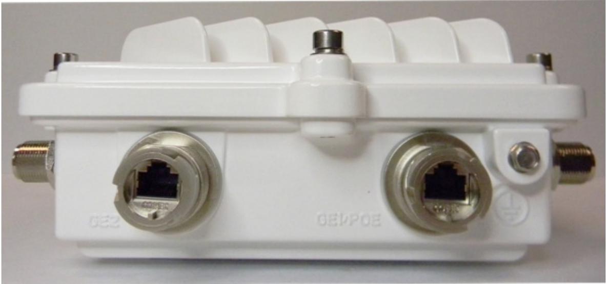
The Ethernet cable from the PoE device (if used) connects to the GE1/POE port on the unit.
