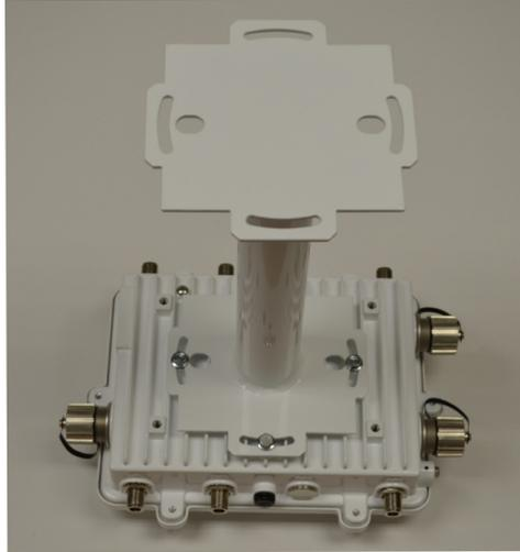
2. Attach the extension arm directly to the wall with lag bolts for other appropriate fasteners.
