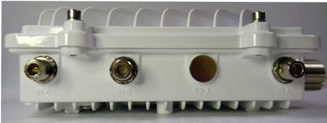
When mounting antennas to ports R1-A, R1-B, and R1-C, ensure that you have selected the appropriate band for the configured radio that uses ports R1-A, R1-B, and R1-C. In this instance, R1 ports relate to the software configured radio 1 settings.
