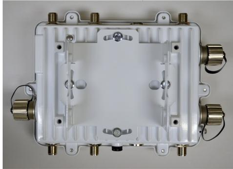
4. Insert two M6 hex flange screws into the bottom holes on the sides of the Access Point bracket section.
