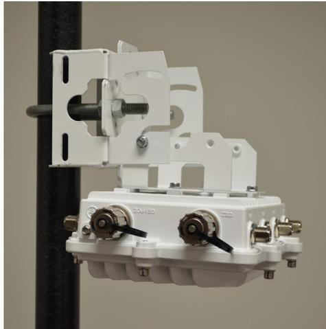
7. Rotate the Access Point bracket section upward and align the top holes on the sides with the top holes on the angle adapter bracket section. Insert two M6 hex flange screws into the top holes on the angle adapter bracket section.
