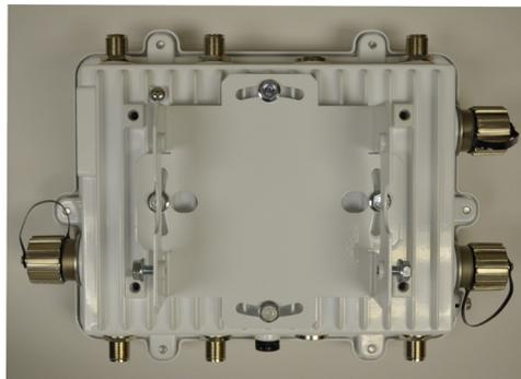
3. With the Access Point positioned so that the gore vent is facing down, insert the two M6 hex flange screws in the bottom holes on the sides of the Access Point bracket section into the open slot connections on the bottom of the angle adapter bracket section. Rotate the Access Point bracket section upward and
