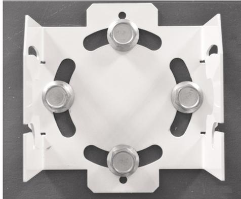
2. Using a torque wrench or a ratchet and a 10mm socket, or an adjustable wrench, attach (but don't tighten) the Access Point bracket section to the AP 7161 with four M6 hex flange screws and insert two M6 hex flange screws into the bottom holes on the sides of the Access Point bracket section.
