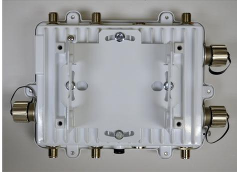
5. Insert two M6 hex flange screws into the bottom holes on the sides of the Access Point bracket section.
