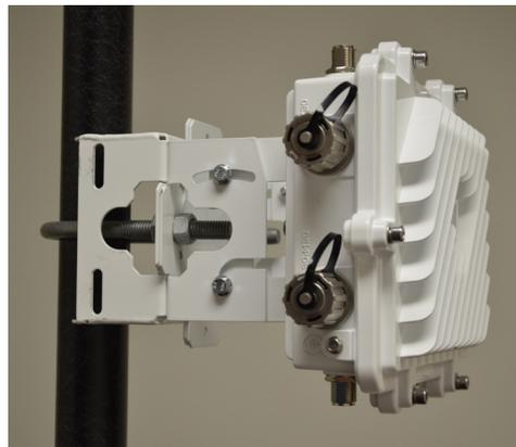
8. Use a torque wrench or a ratchet and a 10mm socket, or an adjustable wrench, to finish attaching the Access Point bracket section to the angle adapter bracket section with the M6 hex flange screws in the open slot connections and the top holes on the angle adapter bracket section. Do not tighten the screws until all rotation and tilt adjustments are complete.
