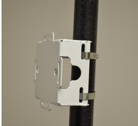
2. With the angle adapter bracket section positioned so that the open connector slots are on the bottom, attach the angle adapter bracket section to the pole mount bracket section using two 1/2 inch bolts and nuts. Tighten the nuts to 30 inch pounds (lbf-in).
