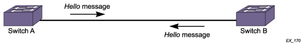
Figure 209: Extreme Networks Switches with ELSM-Enabled Ports Exchanging Hello Messages
