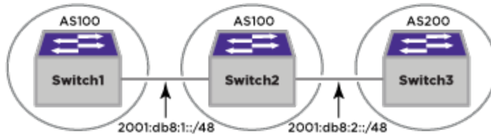
Figure 37: BGP IPv6 Example
