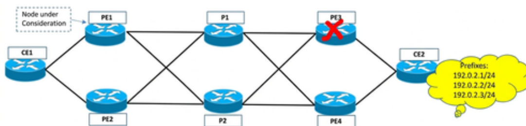
Figure 11: BGP PIC edge node failure
