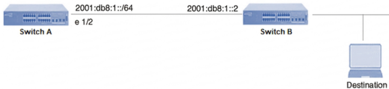
Figure 5: Example of an IPv6 static route
