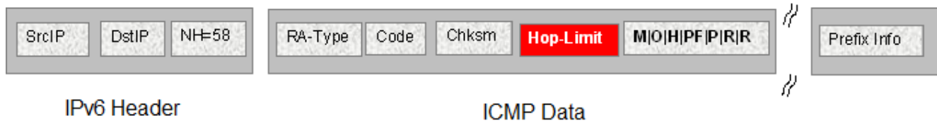
Figure 168: IPv6 ICMP RA data packet outline
