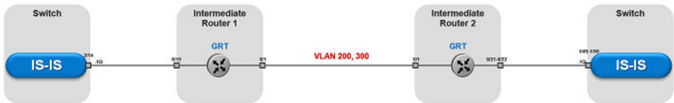
Figure 82: FE over Pseudowire traffic flow component view
