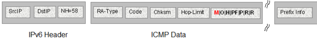
Figure 167: IPv6 ICMP RA data packet outline
