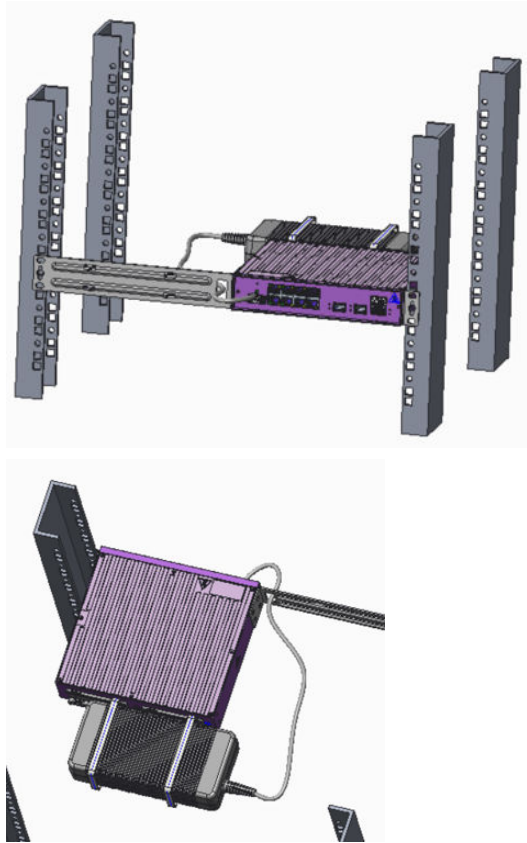
Figure 57: V300-8P-2X Single Rack Mounting with PSU
