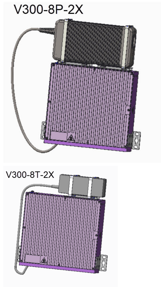
Figure 49: V300-8P/8T-2X Wall Mount with PSU
