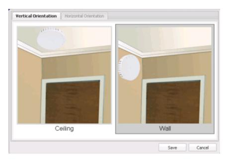
c. If the AP is on a wall, the **Horizontal Orientation** tab appears and allows you to select the approximate direction the AP is facing.
