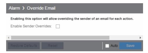
Enable this option to override the sender of an email for an alarm email action, including the ability to set the sender's password, if needed. Since alarms are typically sent out as email/text messages, this option allows IT staff to set different ring-tones based on the alarm definition. Doing this on a smartphone typically involves changing the ring-tone for calls from a specific person.
