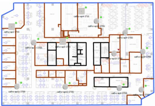
AP. Be sure to place an AP on the correct side of a wall.
