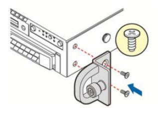
Installing the Rack Handles
