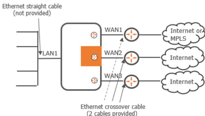
1. Install the appliance between your WAN router(s) and the LAN as shown in the diagram.
