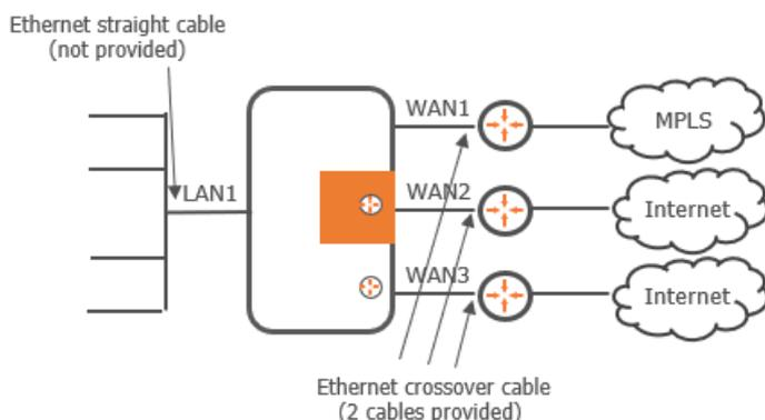
1. Install the appliance between your WAN router(s) and the LAN as shown in the diagram.
