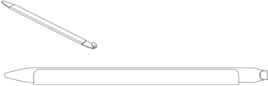
Figure 25: Optical transceiver extraction tool
