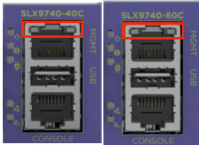
Figure 38: 1 Gb RJ45 Management Port LEDs
