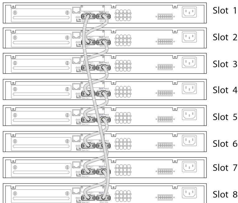
Figure 222: SummitStack Cable Connections Using Eight Switches with Integrated SummitStack Ports
