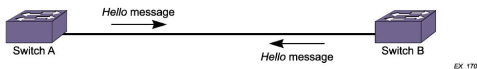
Figure 201: Extreme Networks Switches with ELSM-Enabled Ports Exchanging Hello Messages
