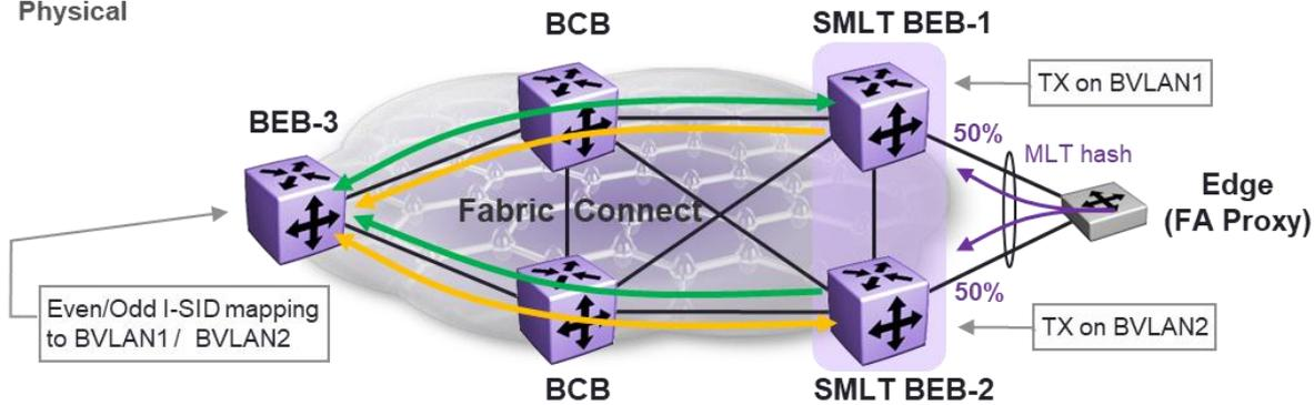
Figure 90 L2 VSN Load Balancing into SPB Equal Cost Shortest Paths
