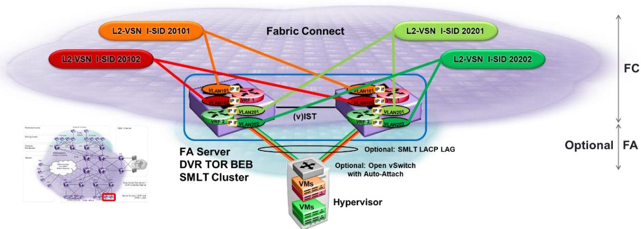
Figure 84 Data Center Top of Rack (ToR) BEB with SMLT clustering
