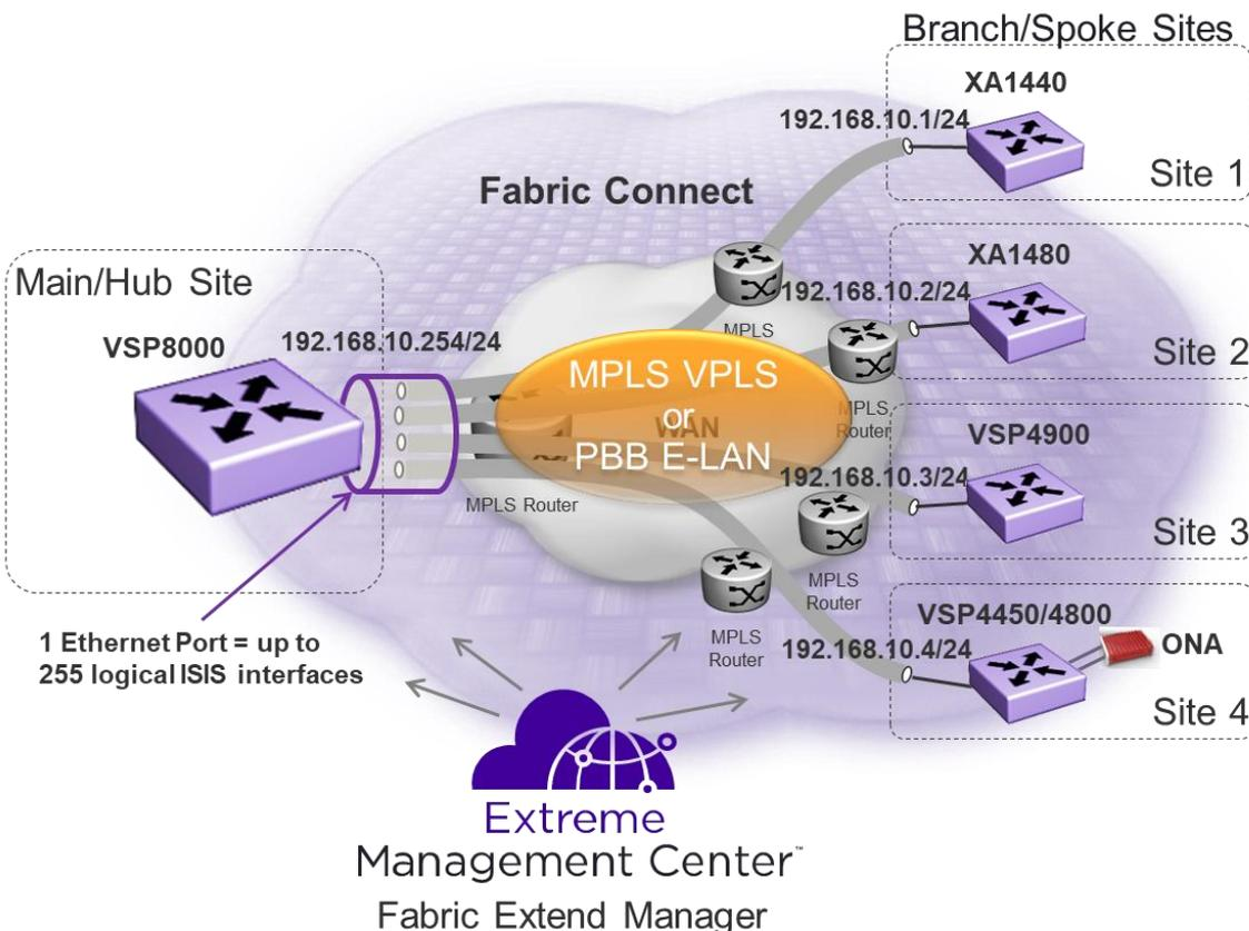
Figure 58 Fabric Extend over WAN L2 Any-to-Any E-LAN Service
