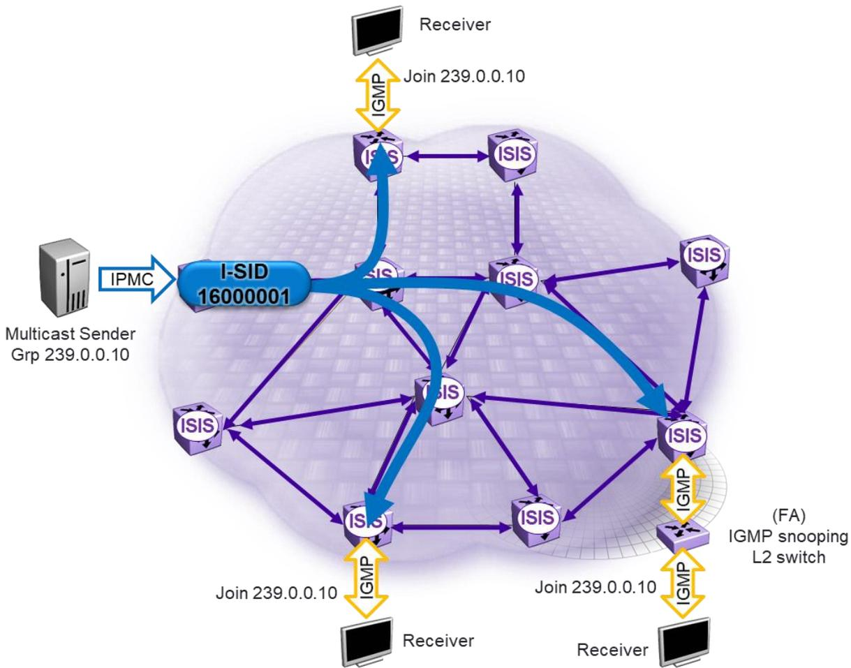
Figure 45 IP Multicast with SPB
