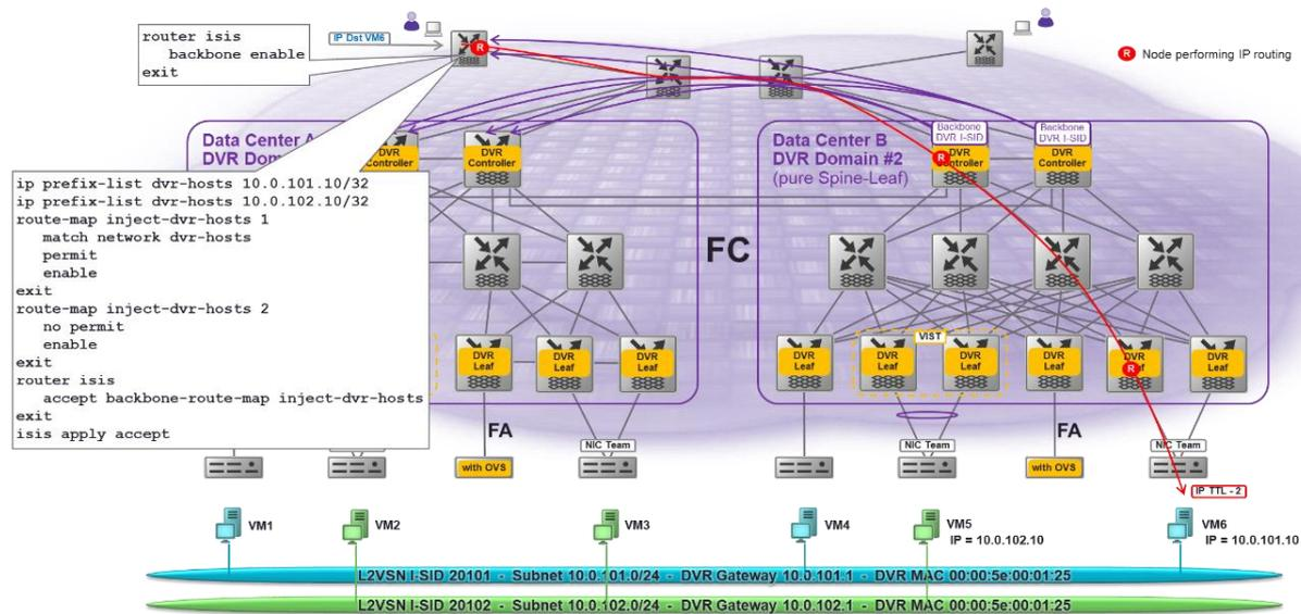
Figure 73 Eliminating North-South Tromboning with DVR, Over Campus Fabric
