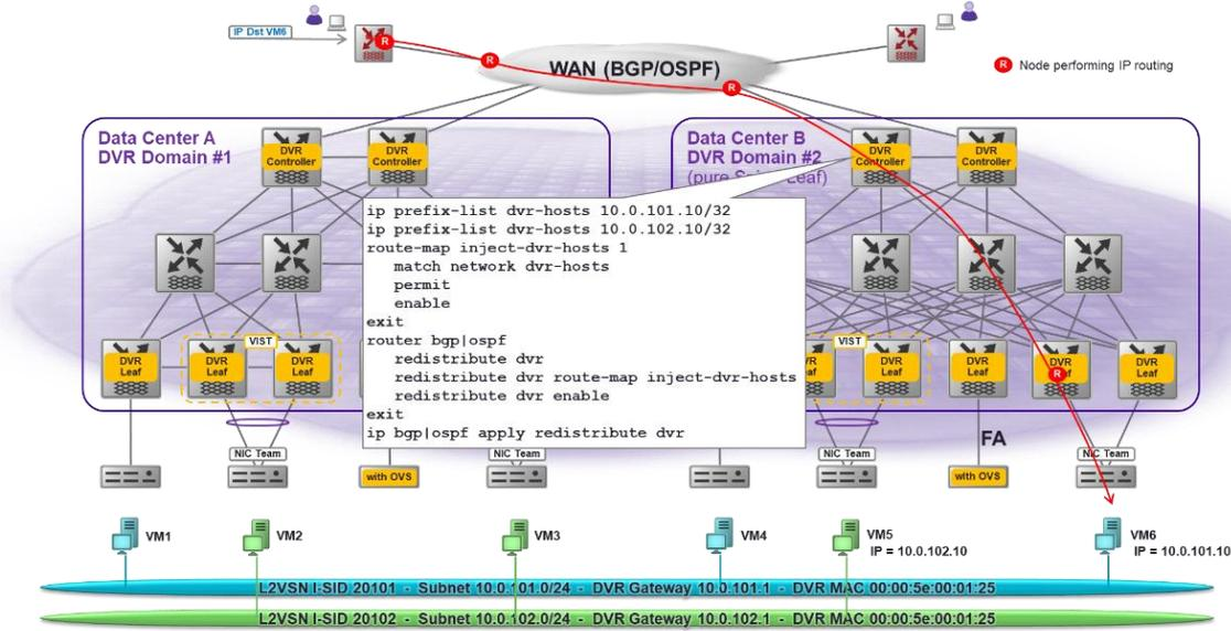
Figure 74 Eliminating North-South Tromboning with DVR, Over Legacy WAN
