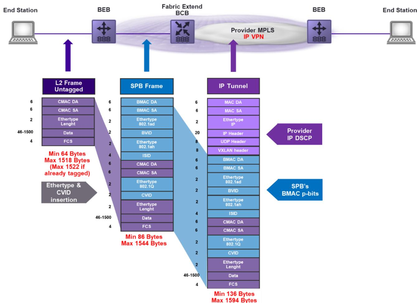
Figure 80 QoS Marking Over Fabric Extend
