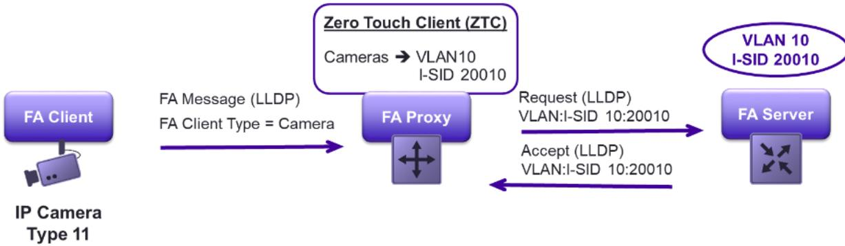
Figure 39 FA Zero-Touch-Client Assigns VLAN:I-SID Binding to Discovered FA client
