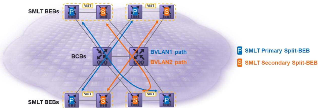
Figure 22 SPB shortest path optimization via SMLT Primary/Secondary BEB positioning
