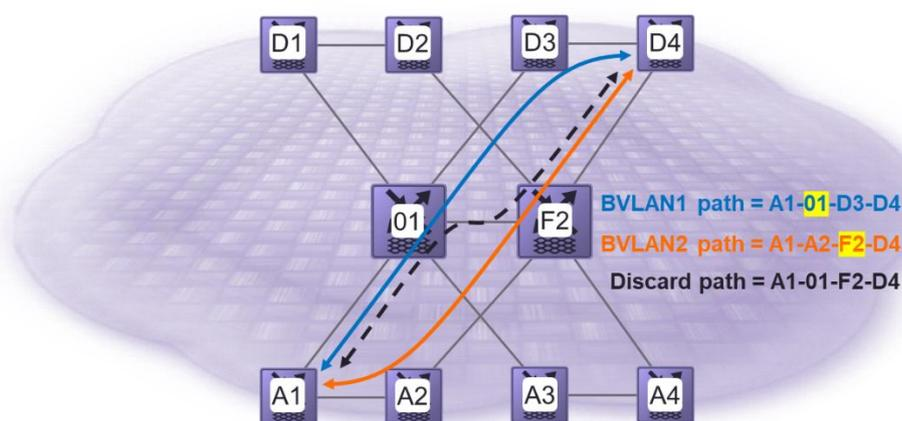
Figure 21 Example of SPB's ECT algorithms to select shortest paths
