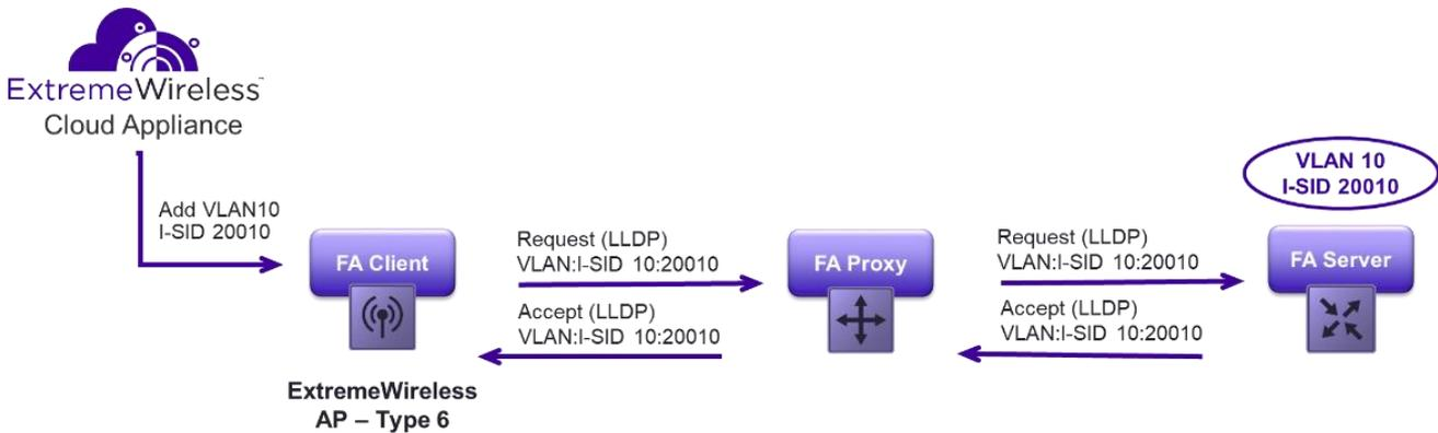
Figure 38 FA Client Requests VLAN:I-SID Binding
