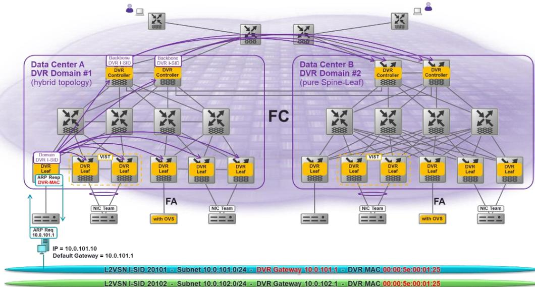
Figure 68 DVR’s Distributed Anycast Gateway in Action
