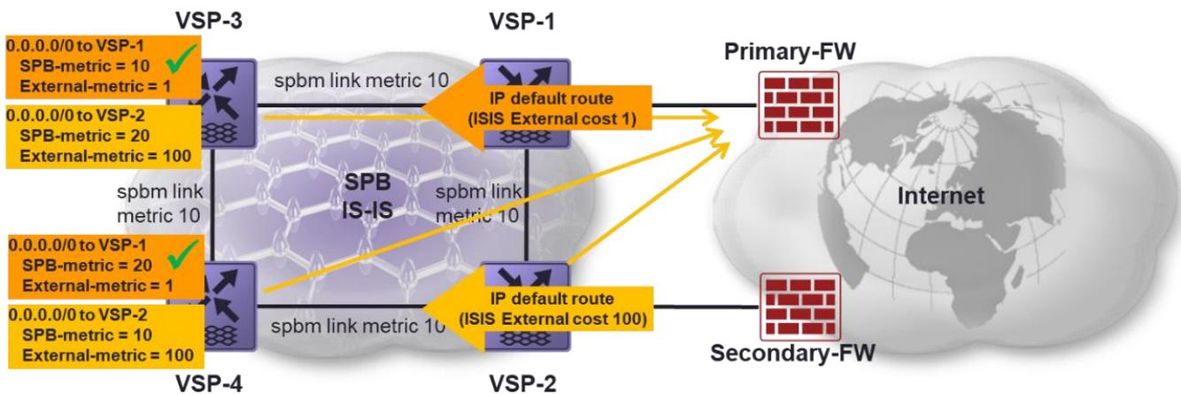
Figure 27 IS-IS External Routes Prefer Lower Route Metric over SPB’s Shortest Path
