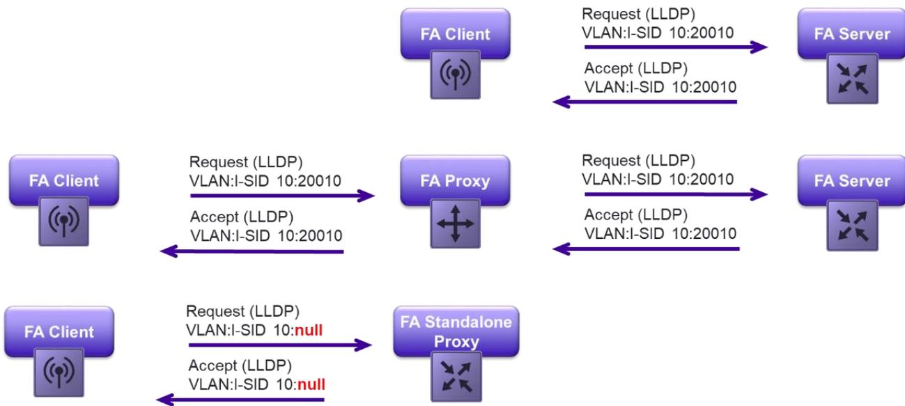
Figure 35 Fabric Attach Model
