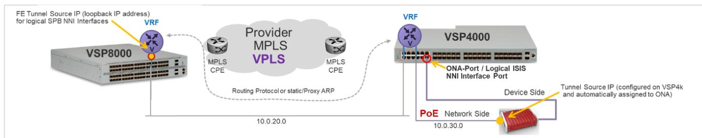
Figure 59 Fabric Extend Deployment Model over WAN L2 E-LAN Service
