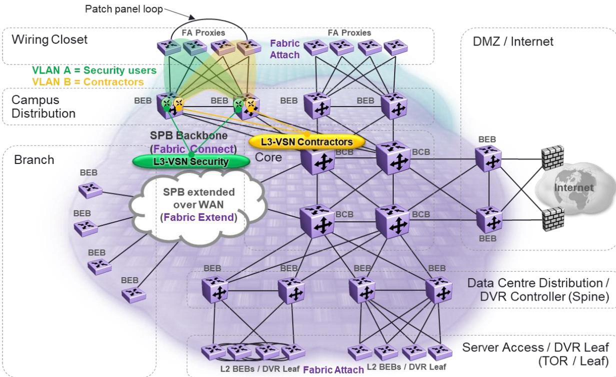
Figure 93 Access VLANs Collapsed Together
