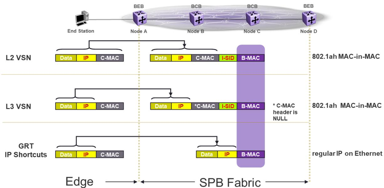
Figure 23 Different Encapsulation Used by GRT IP Shortcuts
