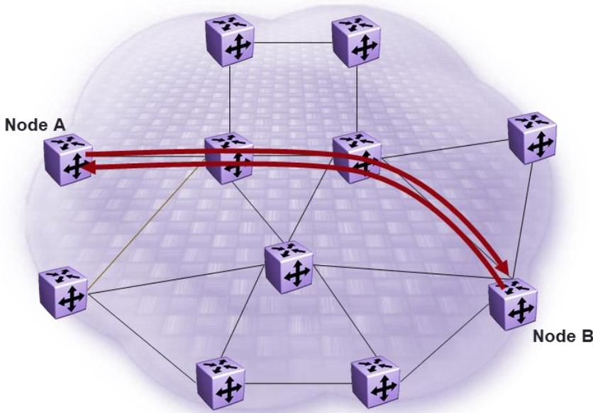
Figure 18 Unicast Shortest Path Between Two Nodes; Forward & Reverse Congruent
