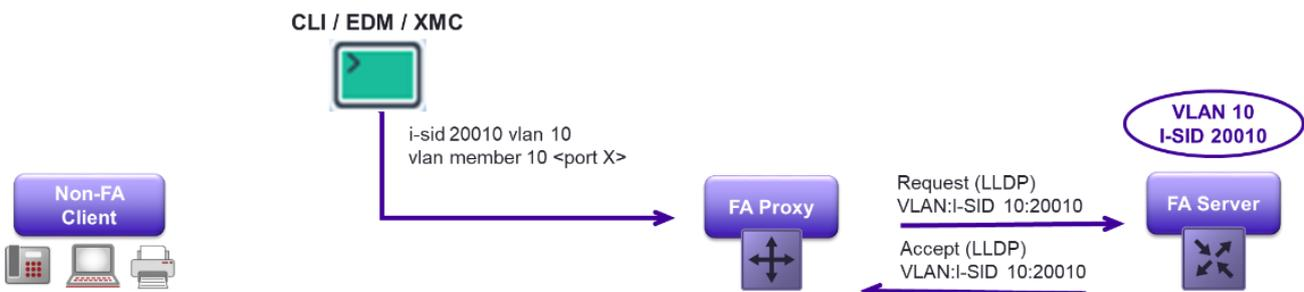
Figure 41 VLAN:I-SID Binding via Manual Configuration
