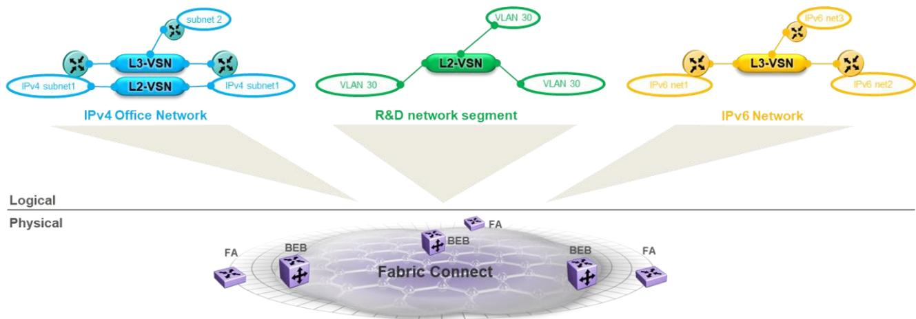
Figure 7 Virtualization of Logical Networks over SPB
