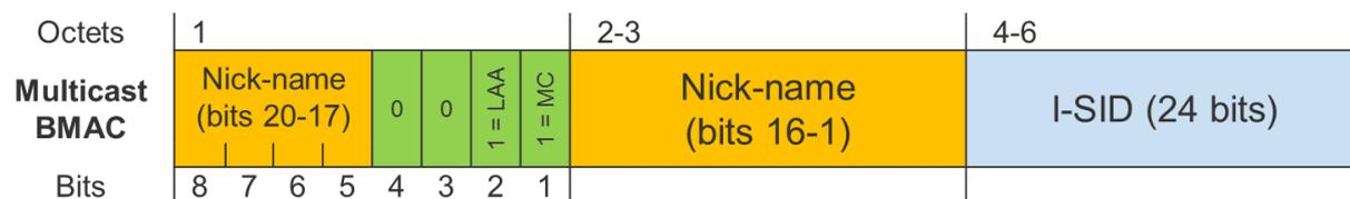
Figure 15 How the SPBM Nick-name is Used to Construct a Multicast BMAC
