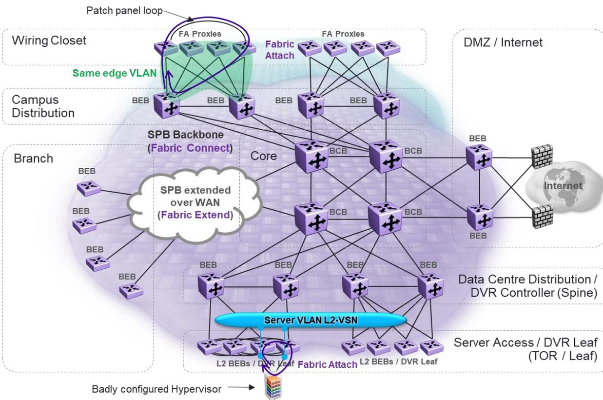
Figure 92 Loop Forming on Access VLAN
