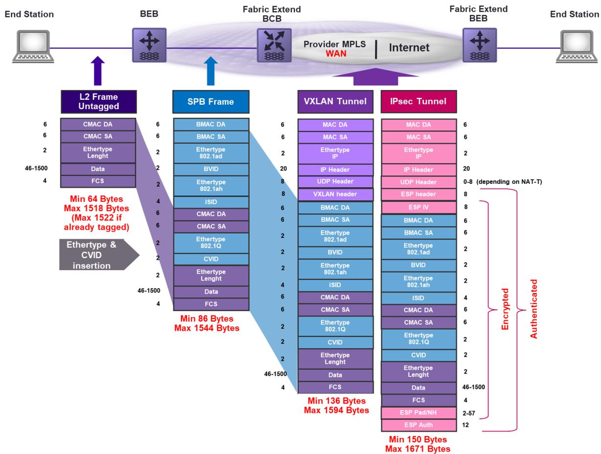
Figure 53 Fabric Extend IP Mode (VXLAN / IPsec) MTU Considerations
