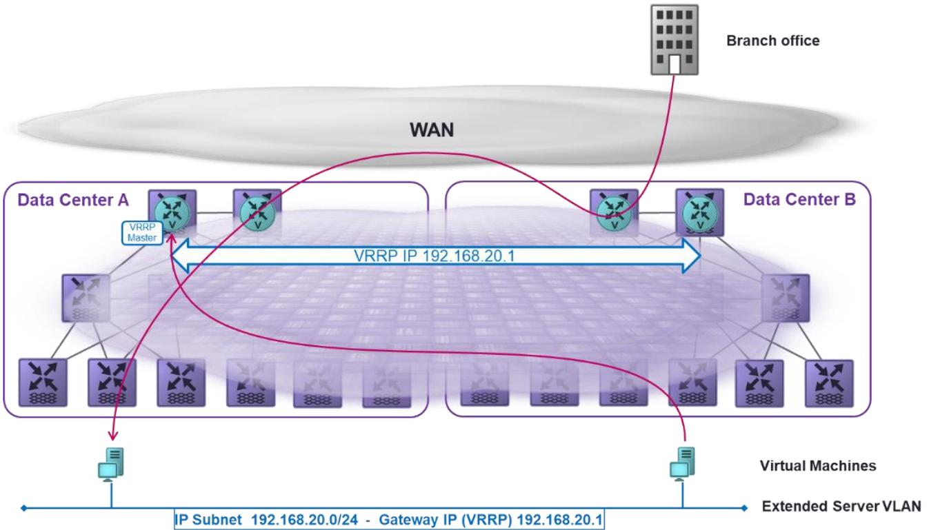
Figure 64 Traffic Tromboning Challenges in a Non-DVR Enabled Data Center
