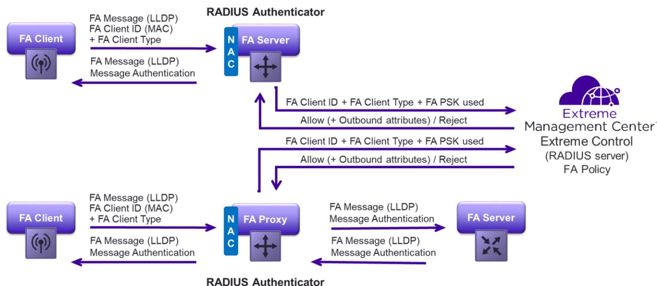
Figure 43 FA Message Authentication Hardening RADIUS MAC-Based Authentication
