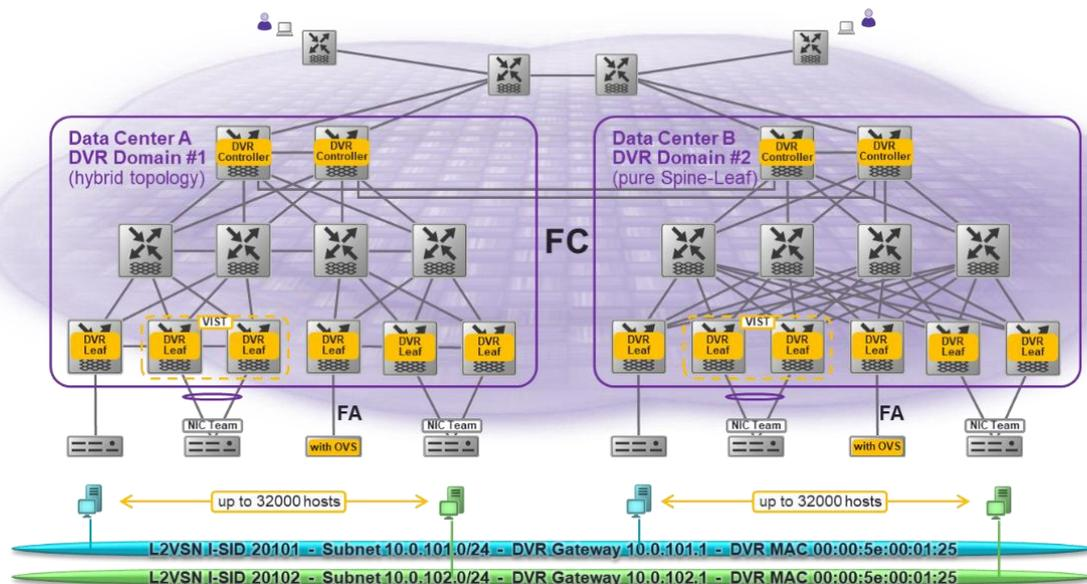
Figure 5 Data Center Virtualization with SPB and DVR
