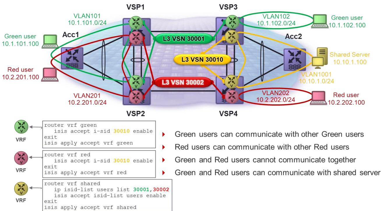
Figure 26 Simplicity of Using IS-IS Accept Policies with SPB
