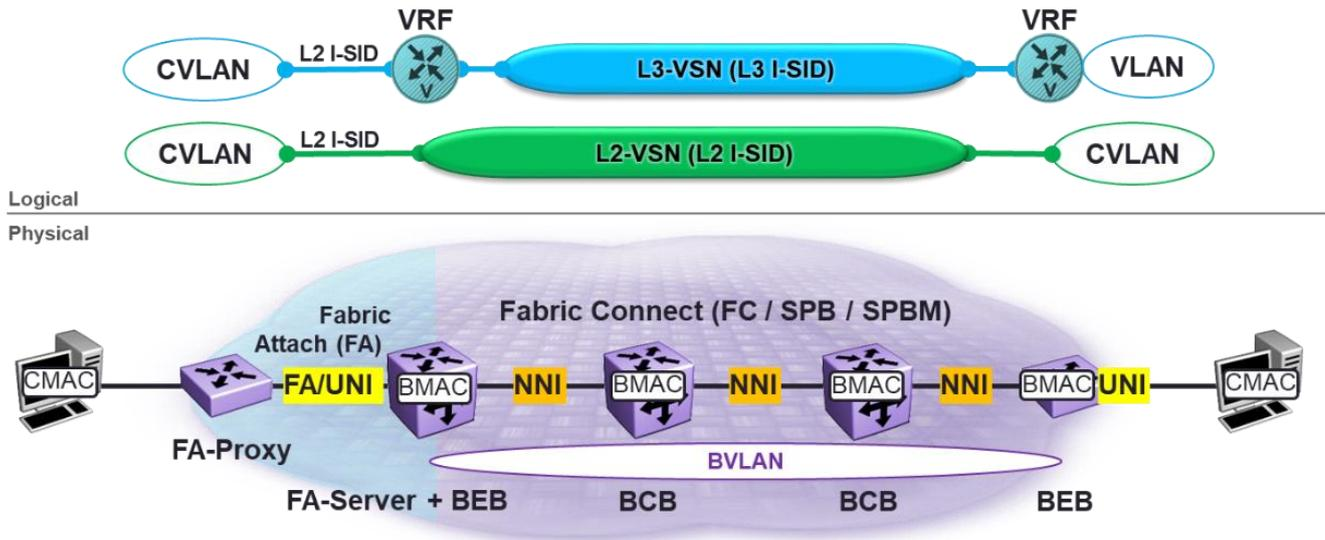
Figure 13 SPB Fabric Architecture Components
