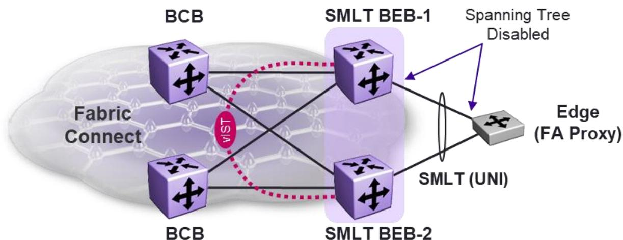
Figure 86 Split Multi-Link Trunking (SMLT) Used in SPB Fabric Access
