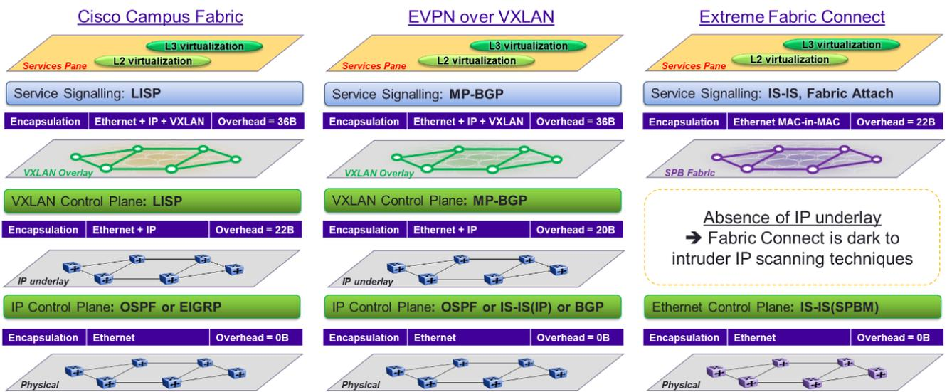
Figure 6 Overview of Fabric Layers and Overlays
