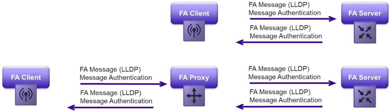
Figure 42 Fabric Attach Message Authentication
