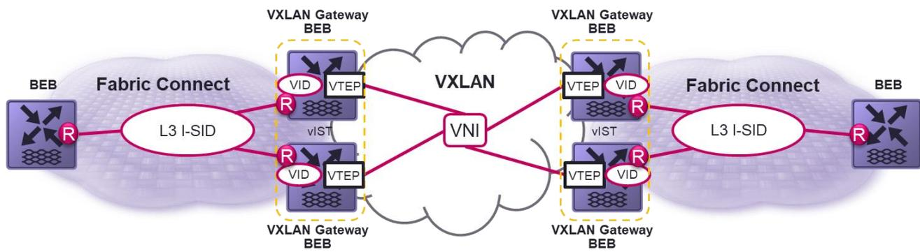
Figure 63 Extending an L3 VSN across Fabrics with VXLAN Gateway
