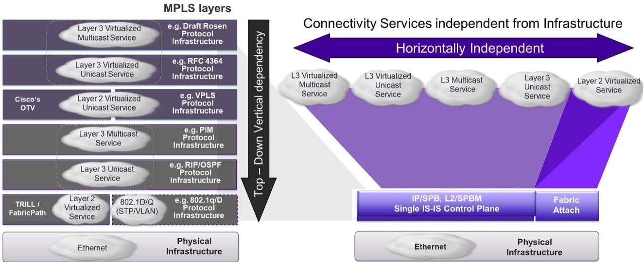
Figure 2 Comparison of SPB’s Simplicity with Traditional Protocol Stack
