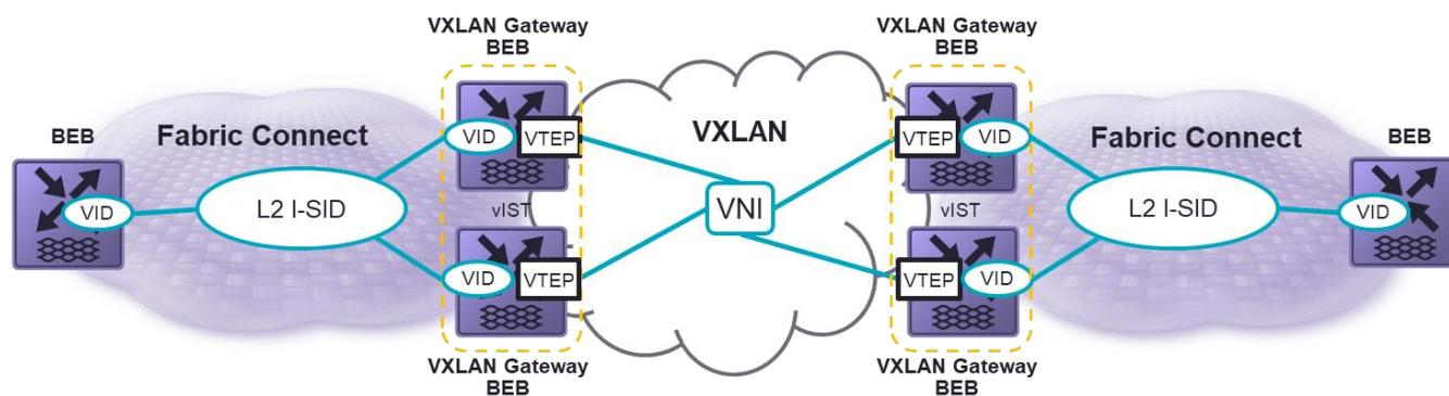
Figure 62 Extending an L2 VSN Across Fabrics with VXLAN Gateway
