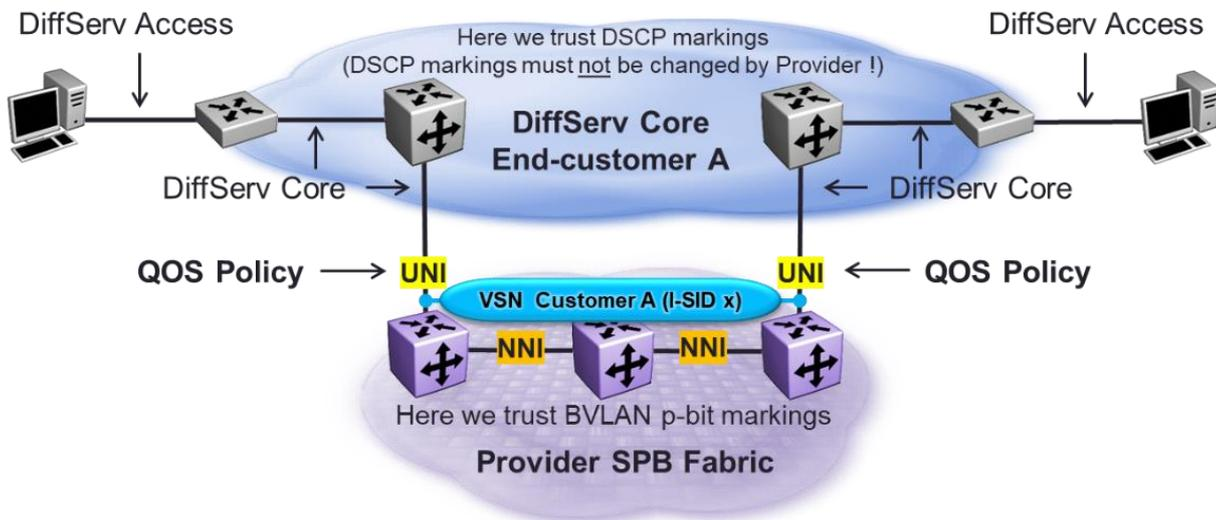
Figure 78 SPB QoS Provider Model
