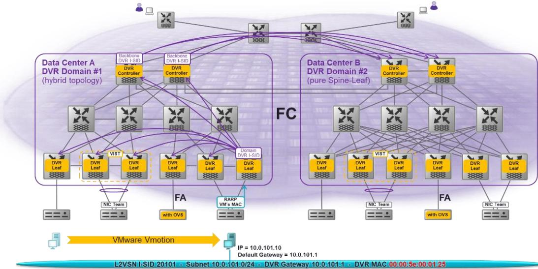
Figure 70 DVR Using RARP with VMware Vmotion
