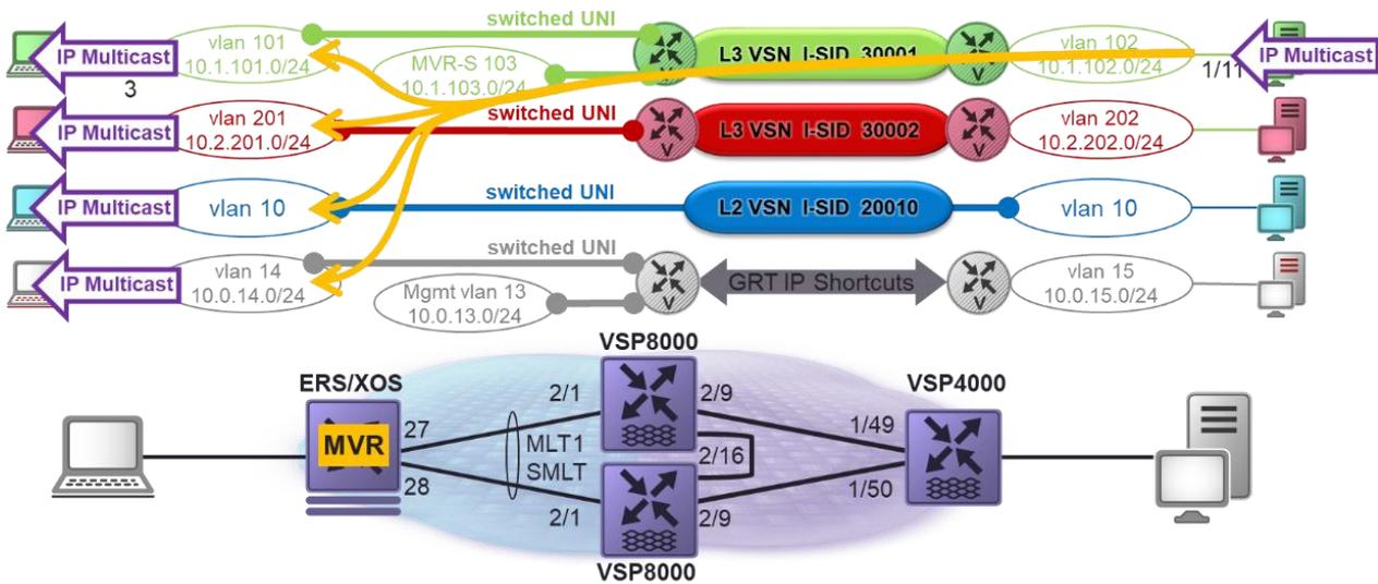
Figure 49 Inter-VSN IP Multicast with MVR on FA Proxy
