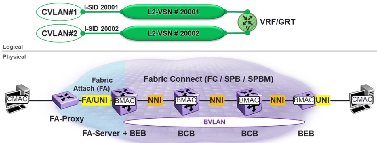
Figure 16 SPB Fabric Inter-VSN Routing
