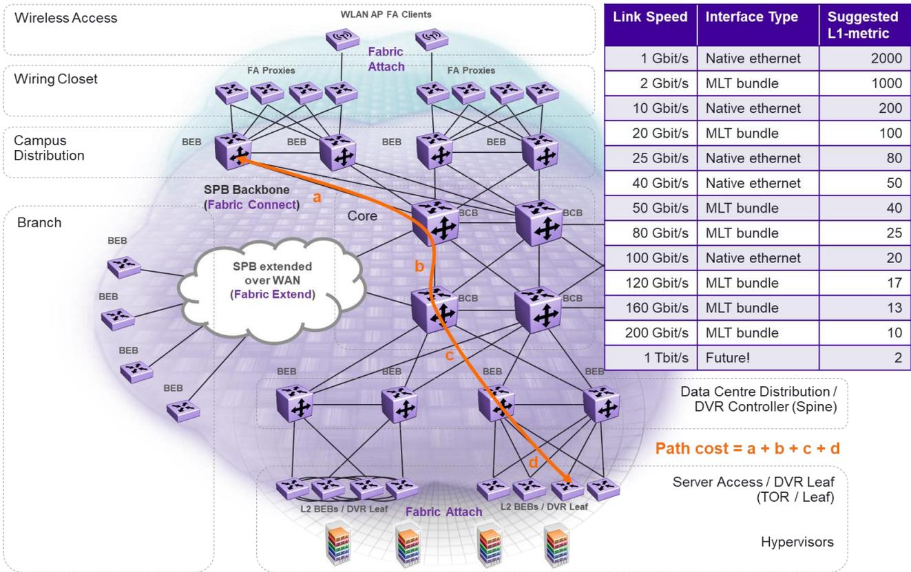
Figure 20 SPB path calculation and suggested link metrics
