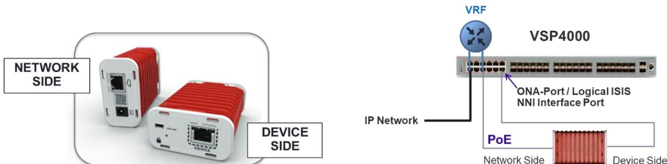
Figure 52 Fabric Extend Pairing of ONA with VSP4000
