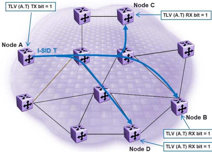
Figure 19 Service-Specific (I-SID) Multicast Shortest Path Tree Rooted at Node A
