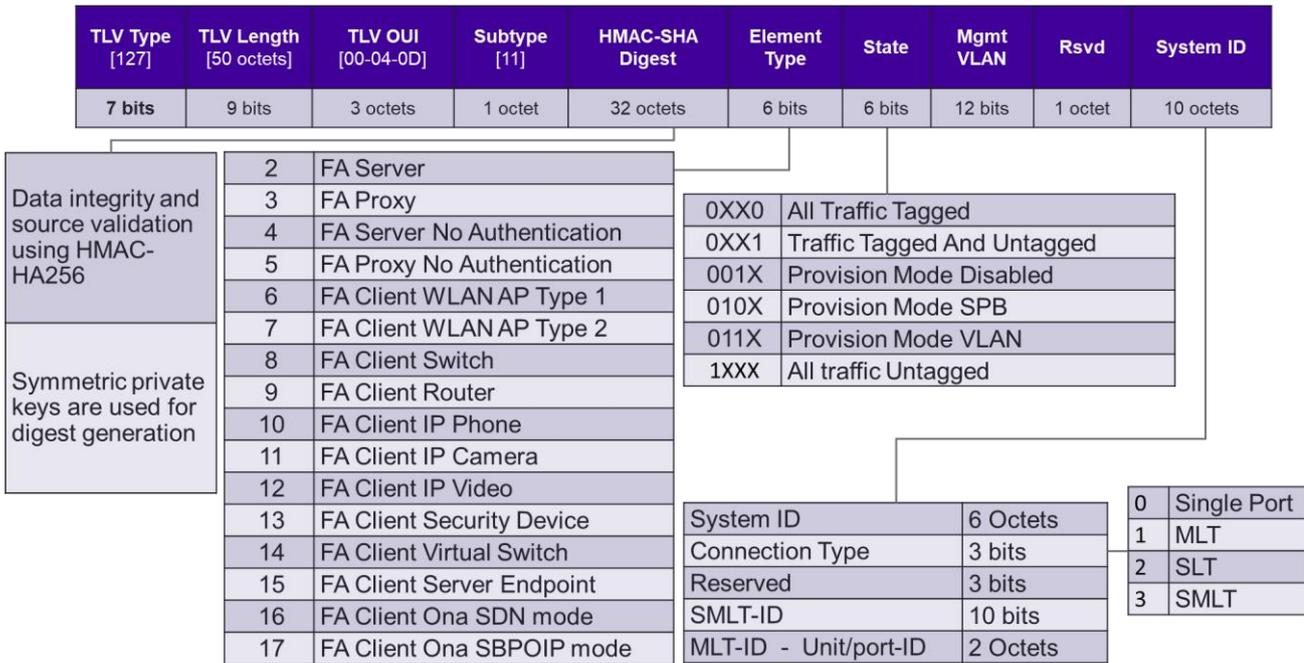
Figure 36 Fabric Attach LLDP Element Signalling TLV
