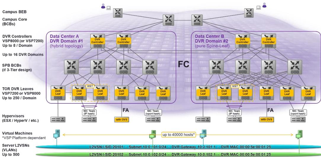
Figure 65 DVR Model and Scaling
