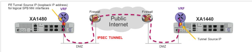
Figure 57 Fabric Extend Deployment Model over Public Internet with IPsec
