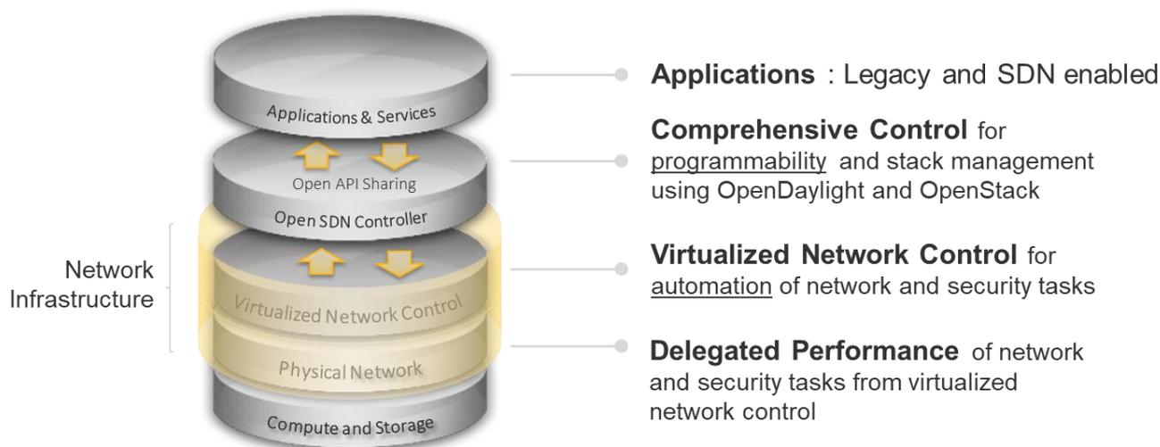
Figure 101 Orchestration of Applications and Services at Cloud Scale
