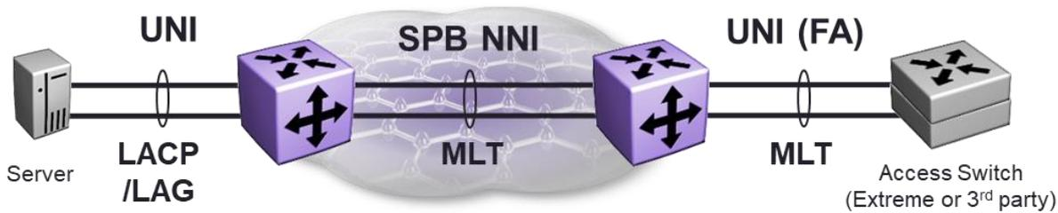
Figure 85 Multi-Link Trunking (MLT) Used in Core and Access
