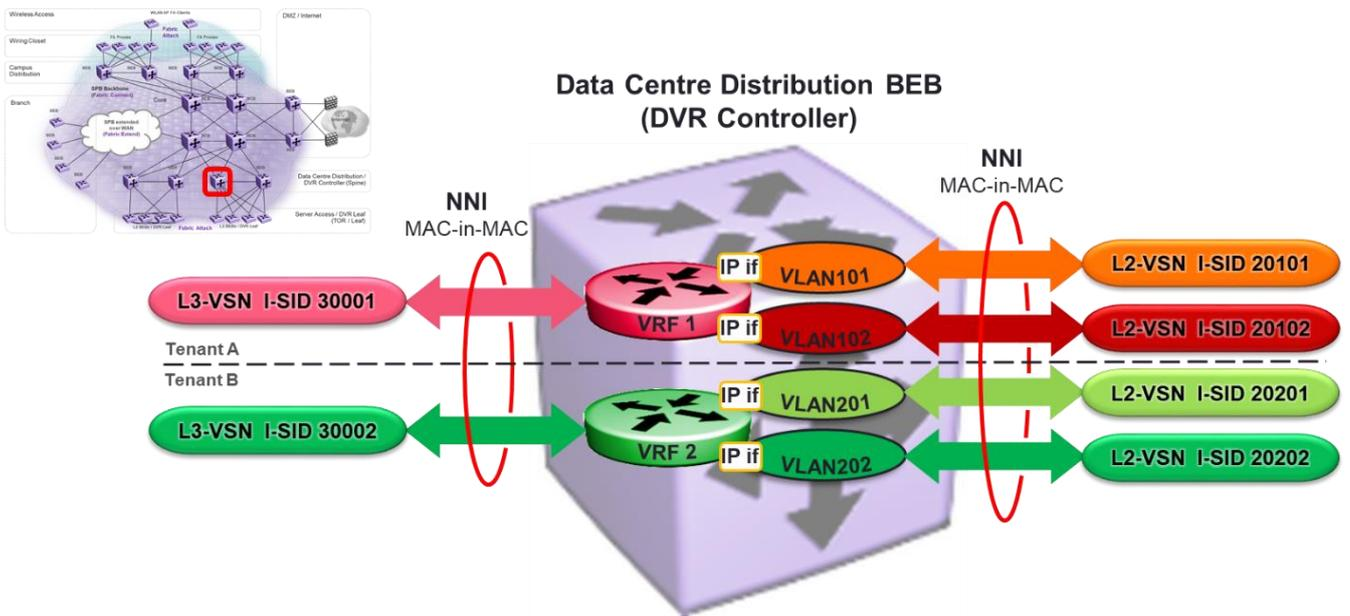
Figure 83 Zoom on Data Center Distribution BEB / DVR Controller
