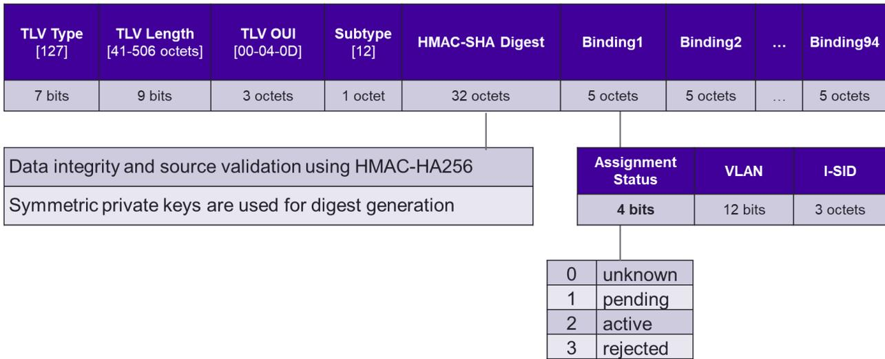
Figure 37 Fabric Attach LLDP Service Signalling TLV
