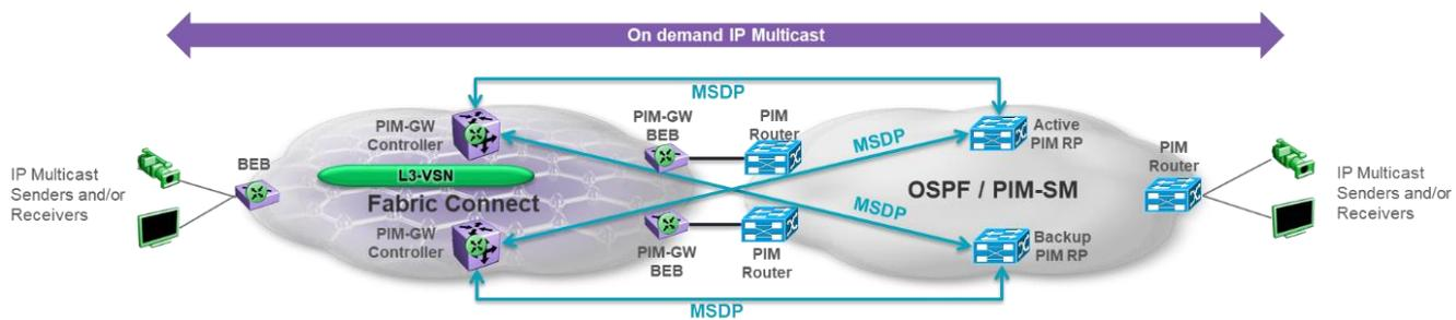
Figure 48 Redundant PIM Gateway Deployment Model
