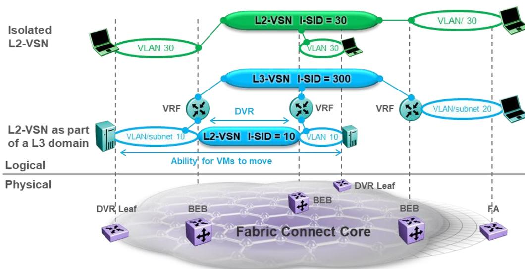
Figure 4 L2 Virtualization with SPB L2 VSNs
