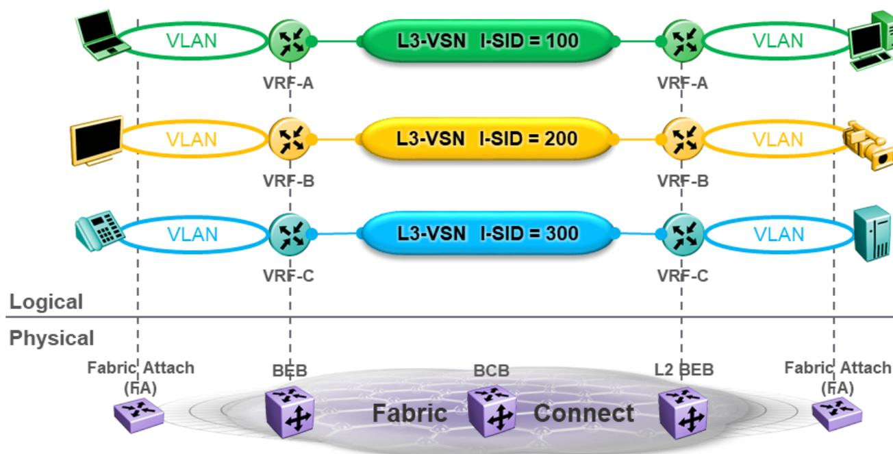
Figure 3 Virtualization with SPB L3 VSNs
