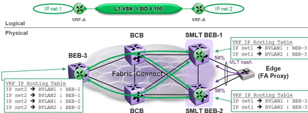
Figure 89 L3 ECMP Translation into SPB Equal Cost Shortest Paths
