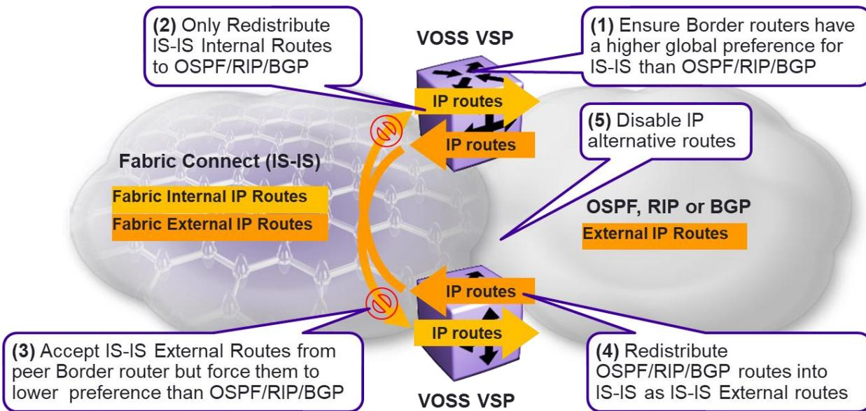
Figure 28 Redundantly IP Routing Fabric VSN with External OSPF/RIP/BGP Network
