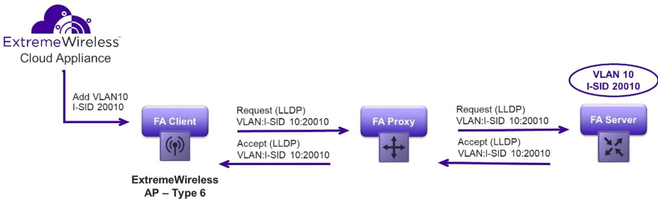
Figure 38 FA Client Requests VLAN:I-SID Binding
