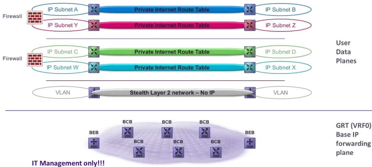
Figure 96 Isolation of the Global Routing Table (VRF0)
