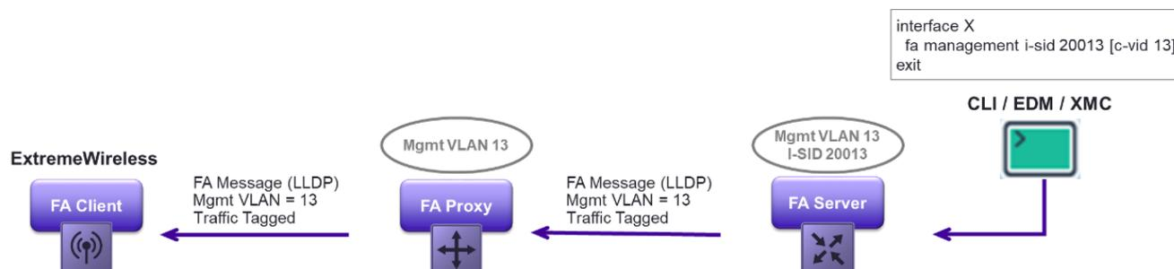
Figure 44 FA Signalling of Management VLAN from FA Server
