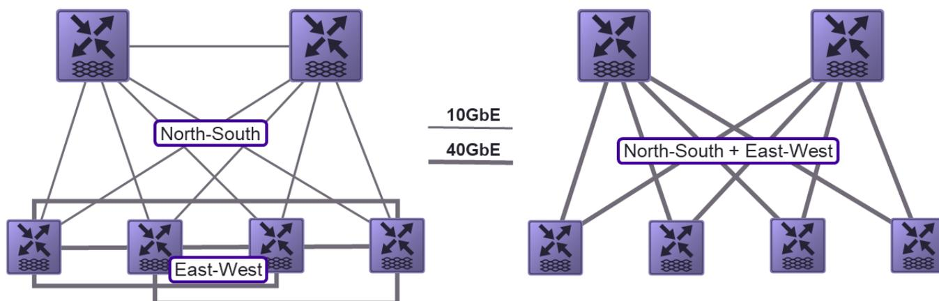
Figure 10 Smaller (Meshed) vs Larger (Spine-Leaf) Topologies
