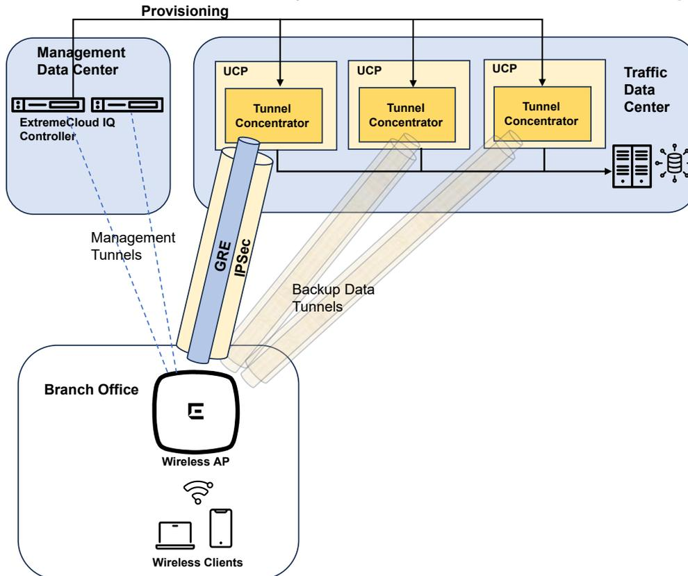
**Figure 2: Tunnel Concentrator Redundancy with ExtremeCloud IQ Controller**
