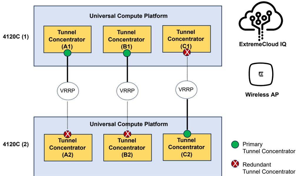
**Figure 3: Tunnel Concentrator Redundancy (with ExtremeCloud IQ)**
