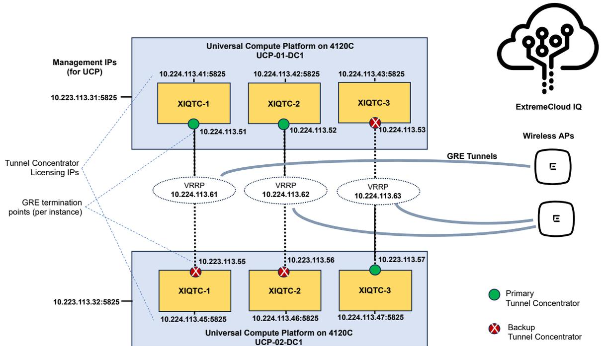
**Figure 4: Configuration Example with ExtremeCloud IQ and Redundancy**
