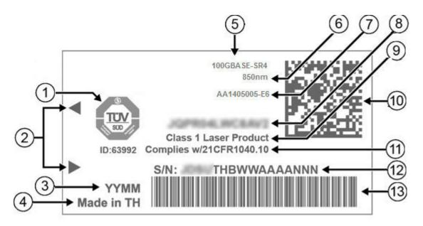
Figure 8: 100GBASE-SR4 QSFP28 transceiver label example
