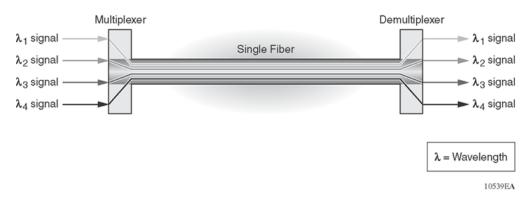
Figure 3: Wavelength division multiplexing
