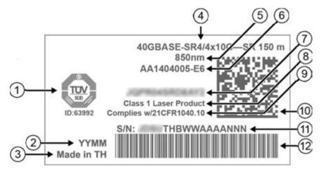
Figure 7: 40GBASE-SR4 QSFP+ transceiver label example
