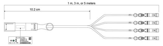
Figure 2: Passive copper BOC
