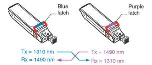
The long wavelength optical transceivers used in these models provide variable distance ranges using single mode fiber optic cabling.
