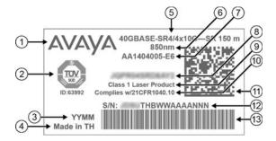
Figure 7: 40GBASE-SR4 QSFP+ transceiver label example
