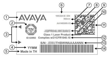
Figure 8: 100GBASE-SR4 QSFP28 transceiver label example
