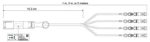
Figure 2: Passive copper BOC
