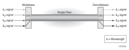
Figure 3: Wavelength division multiplexing
