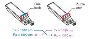
The long wavelength optical transceivers used in these models provide variable distance ranges using single mode fiber optic cabling.
