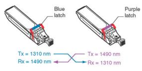
The long wavelength optical transceivers used in these models provide variable distance ranges using single mode fiber optic cabling.
