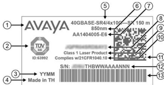
**Figure 7: 40GBASE-SR4 QSFP+ transceiver label example**
