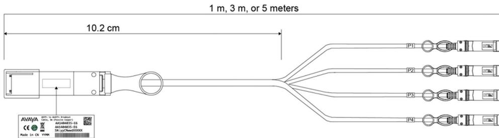
**Figure 2: Passive copper BOC**
