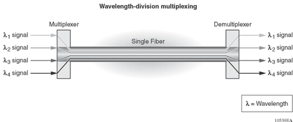
**Figure 3: Wavelength division multiplexing**
