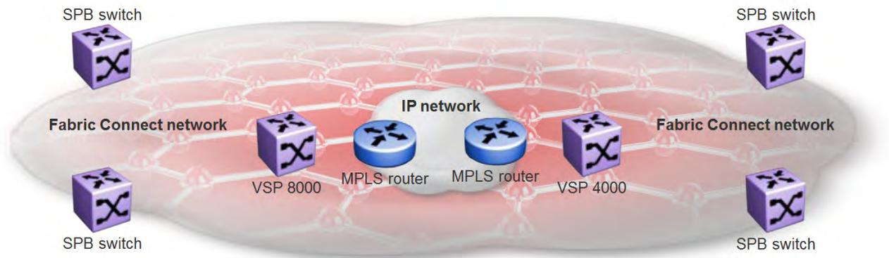
**Figure 6: Single Fabric Connect Domain realized using Fabric Extend**
