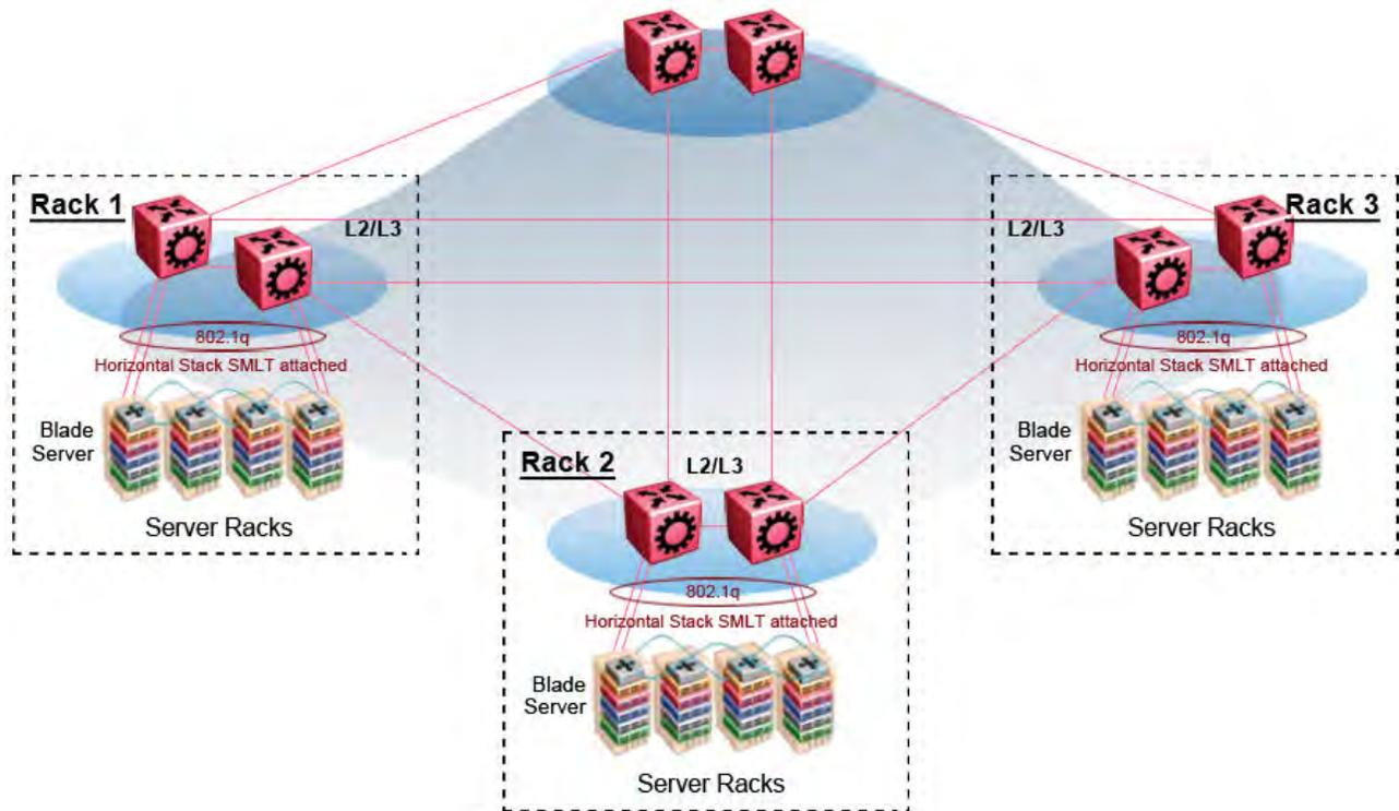
Figure 2: SPBM ring topology with shared data centers
