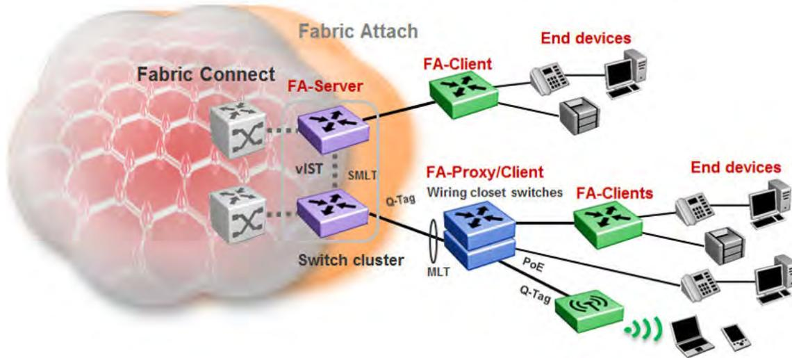
Figure 21: Fabric Attach in a single-homed SMLT deployment
