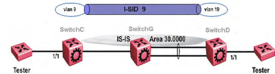
Figure 44: Layer 2 VSN with different VLAN IDs
