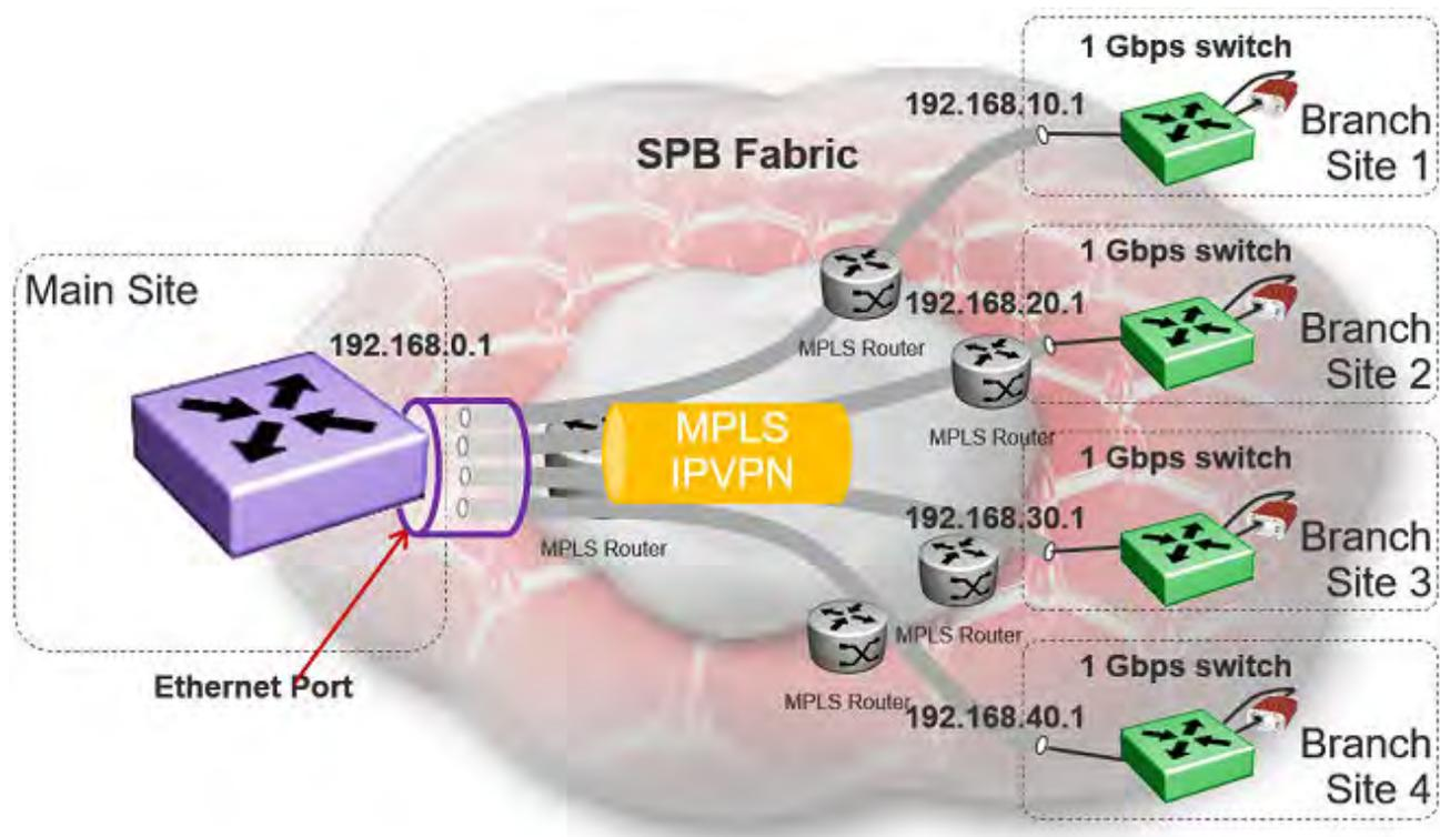
**Figure 9: Fabric Extend IP VPN Deployment Option**
