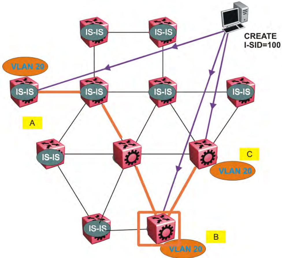
Figure 41: Shortest path tree for source node B
