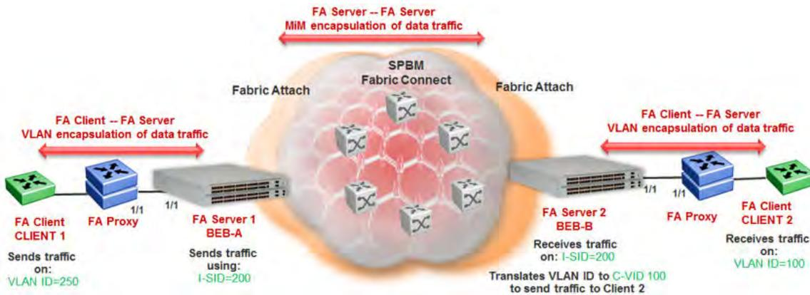
**Figure 18: Data encapsulation — VLAN encapsulation and MiM encapsulation**
