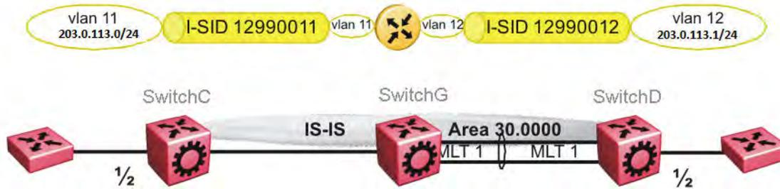
**Figure 46: Inter-VSN routing configuration**
