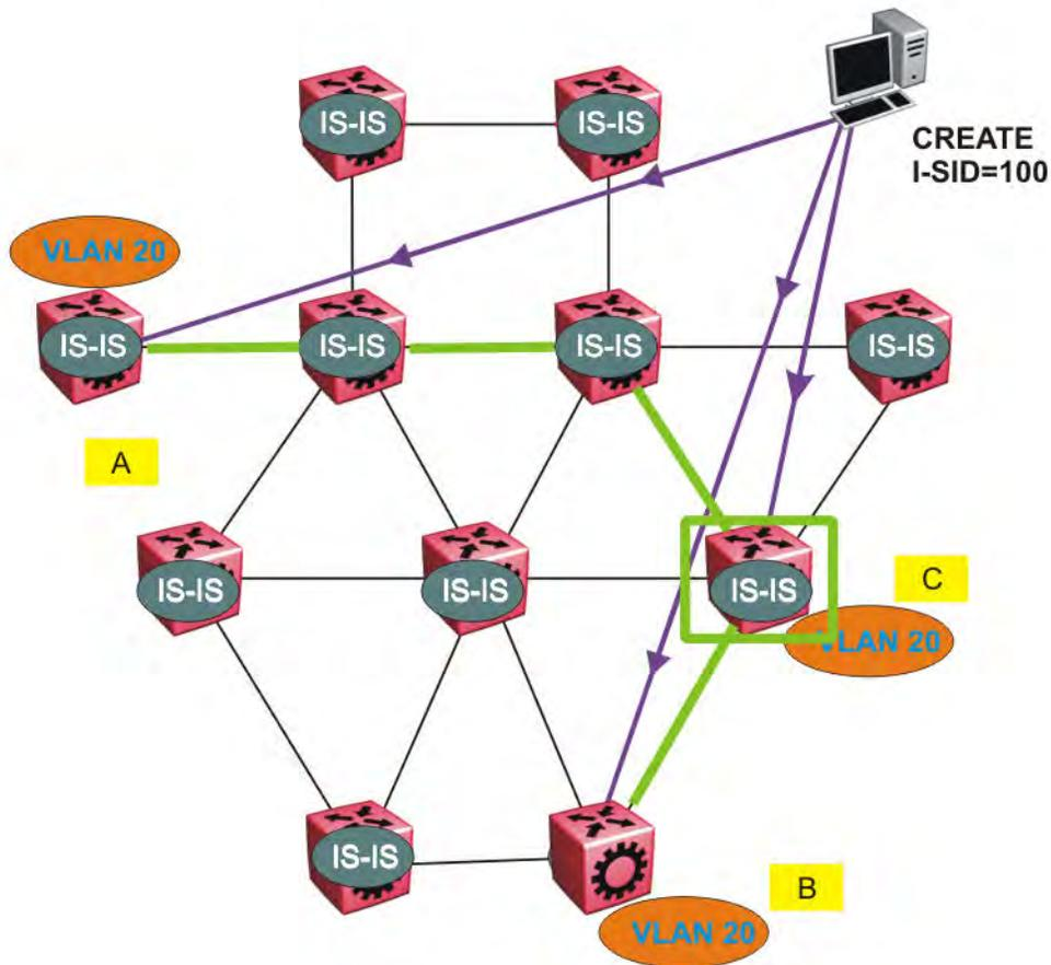
**Figure 42: Shortest path tree for source node C**
