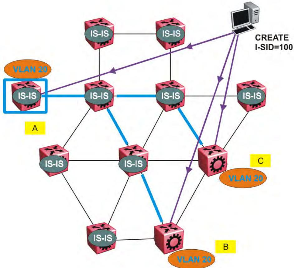
Figure 40: Shortest path tree for source node A
