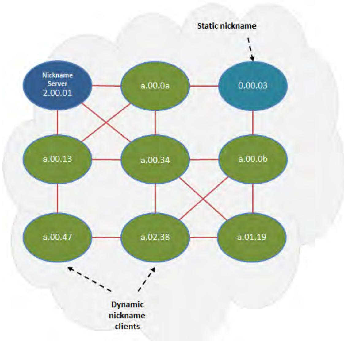
You can configure a node in a FAN as a nickname server. You must configure the nickname server with a static nickname from the nickname allocation range 0.00.01 - 9.FF.FF. The nickname server cannot be started until it is configured with a static nickname. It is recommended that a FAN contain at least two nickname servers to provide redundancy.
