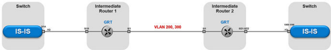
Figure 80: FE over Pseudowire traffic flow component view
