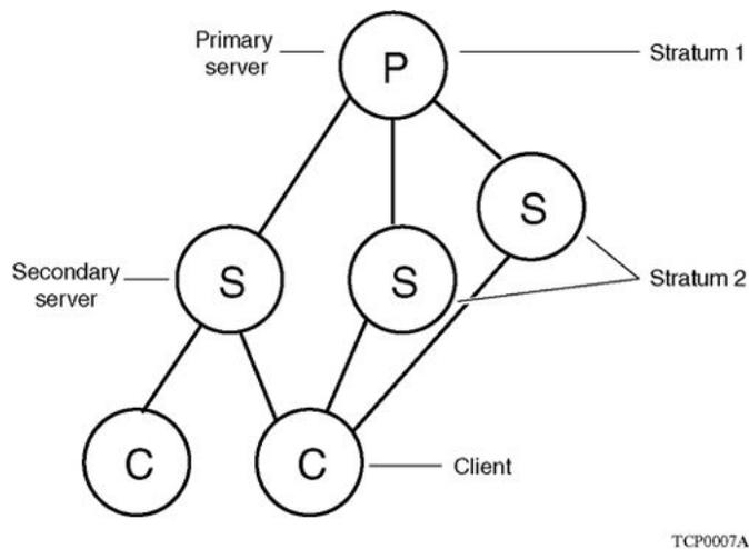
**Figure 3: NTP time servers forming a synchronization subnet**
