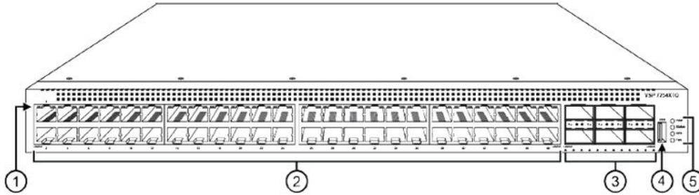
1. LEDs indicating port activity are above the RJ-45 and SFP+ port. The up arrow on the left indicates the top port; the down arrow on the right indicates the bottom port.
