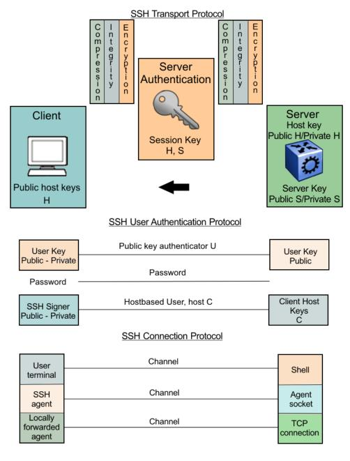
Figure 8: Separate SSH version 2 protocols
