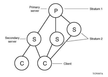
Figure 3: NTP time servers forming a synchronization subnet
