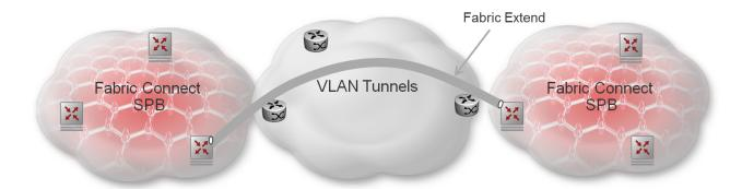
Figure 7: Fabric Extend over VLAN tunnels
