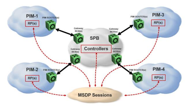
Figure 5: Multicast over Fabric Connect with SPB-PIM GW
