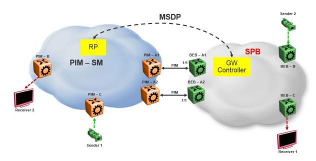
Figure 7: SPB-PIM Gateway base case configuration
