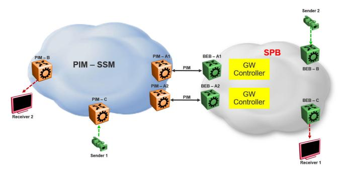
Figure 8: Static configuration of SSM groups in Controllers
