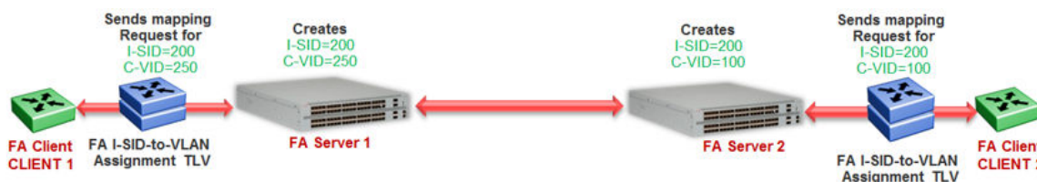
Figure 64: Learning of I-SID-to-VLAN mappings
