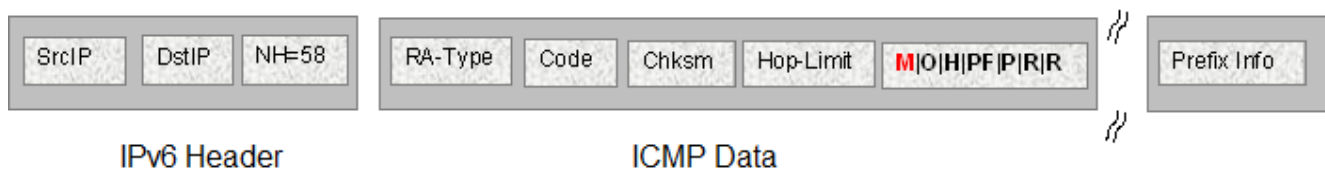
Figure 179: IPv6 ICMP RA data packet outline
