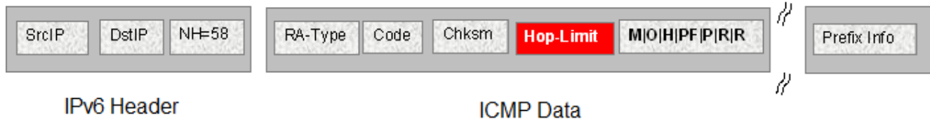
Figure 180: IPv6 ICMP RA data packet outline
