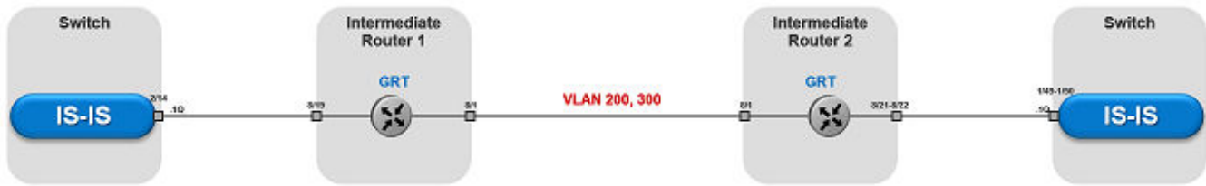
Figure 84: FE over Pseudowire traffic flow component view
