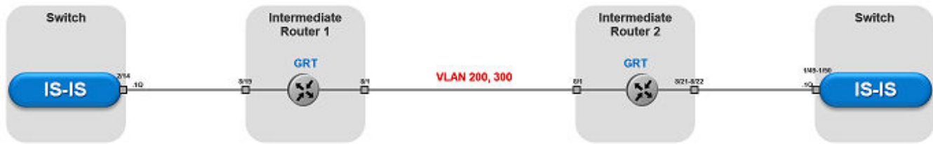
Figure 92: FE over Pseudowire traffic flow component view
