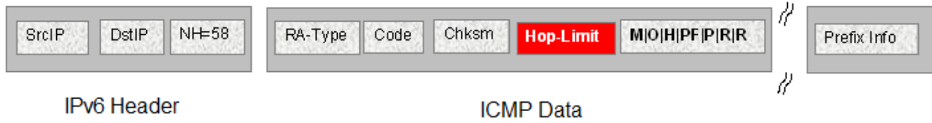
Figure 188: IPv6 ICMP RA data packet outline
