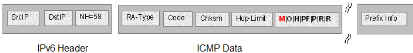
Figure 187: IPv6 ICMP RA data packet outline
