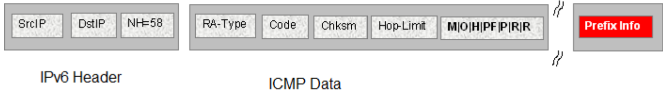
Figure 185: IPv6 ICMP RA Data Packet Outline
