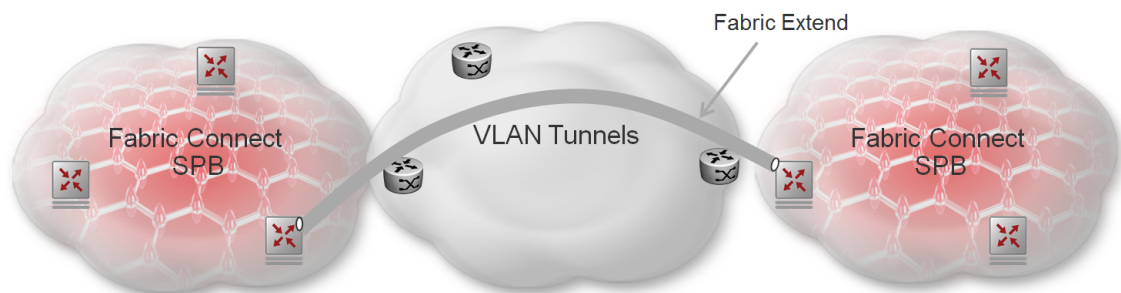
Figure 61: Fabric Extend over VLAN tunnels
