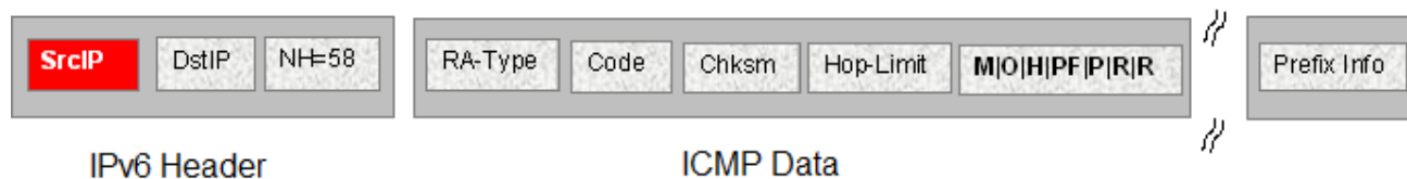
Figure 169: IPv6 ICMP RA Data Packet Outline
