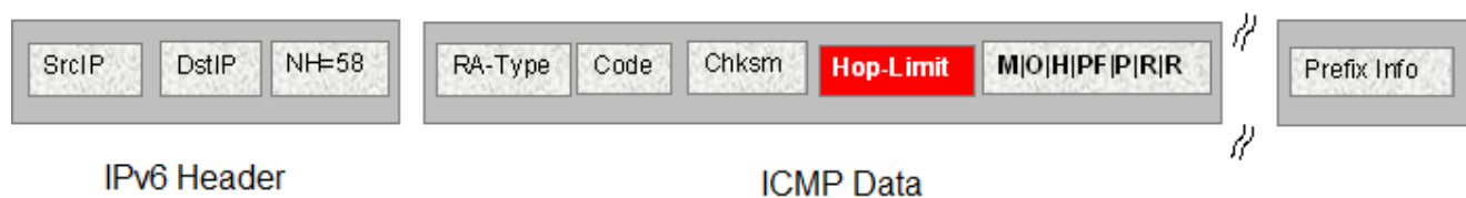
Figure 173: IPv6 ICMP RA data packet outline
